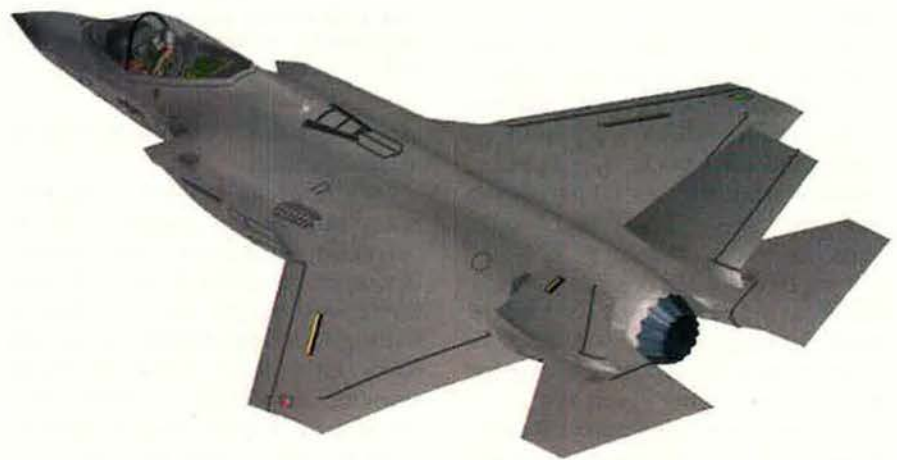
A computer rendering shows the USAF production model. Inlets were moved aft to improve visibility for the pilot, and the overall airplane grew seven inches to permit room for growth in avionics.
