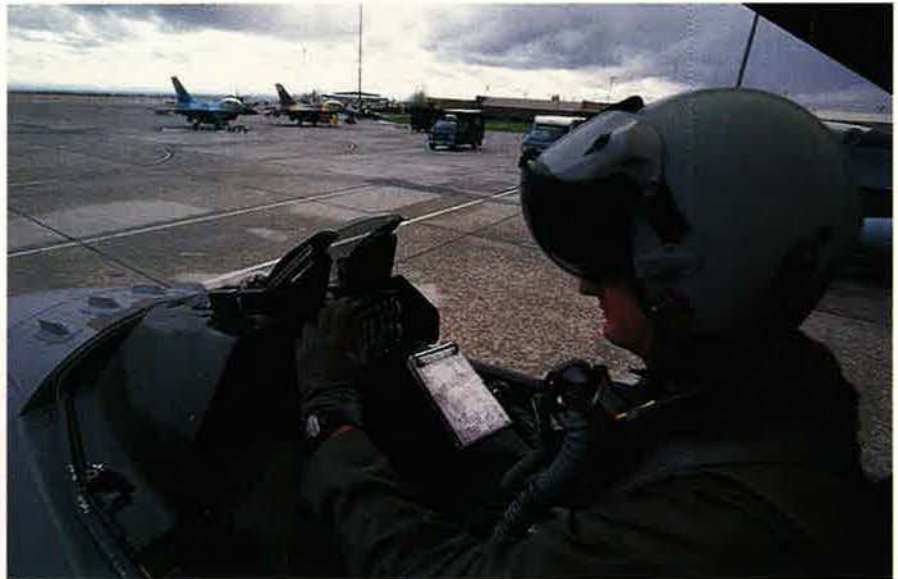
Above, an AIM-9X is visible against a white-tipped AIM-120 AMRAAM, both mounted on an F-15C. At right, an F-16 pilot is wearing the Joint Helmet Mounted Cueing System. JHMCS lets a pilot fire a missile in the direction in which he is looking, not necessarily in the direction the aircraft is flying.
