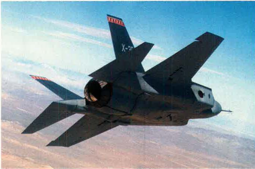
The F-35 will be able to fly with either the Pratt & Whitney F135 engine or General Electric F136 engine. The two power plants, though internally dissimilar, must be interchangeable in size, maintenance, and performance.
