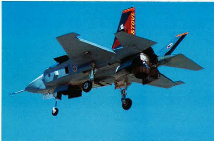
The X-35 STOVL demonstrator accomplished short takeoff, supersonic flight, and vertical landing all in one mission—hence the “hat trick” insignia on the tail.
