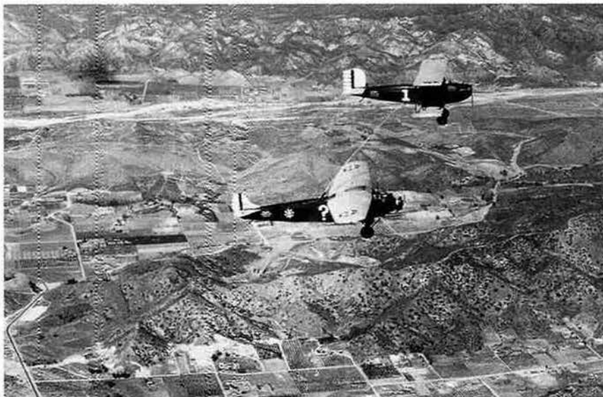
Question Mark's left engine died Jan. 7 when a pushrod failed, so the crew decided to land. All told, Question Mark's crew had hooked up with a refueling aircraft 43 times. Question Mark took on 5,660 gallons of fuel and 245 gallons of oil.
