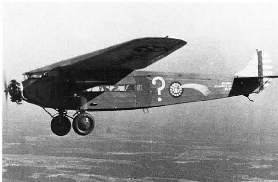
Question Mark was a specially modified Fokker C-2A sporting three powerful and fuel efficient 220-hp radial engines. Modifications included the addition of two 150-gallon fuel tanks as part of the new refueling system.
