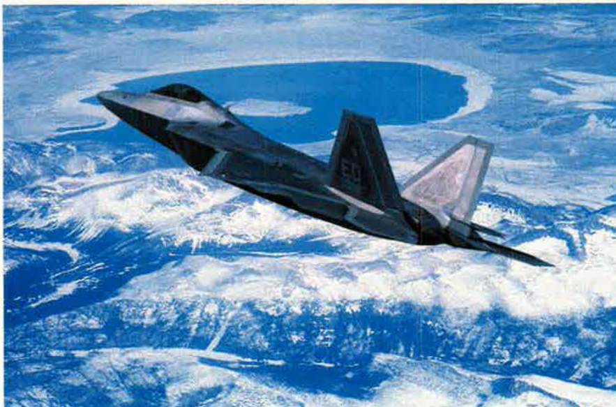
The F/A-22 has unprecedented fighter and attack capabilities. Among its transformational qualities are a balanced design, including stealth, supercruise speed, advanced integrated avionics, and low-observable control surface edges.
