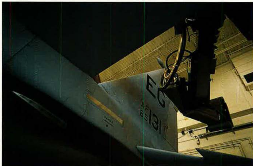
USAF is trying to head off age-related problems. Here, an X-ray machine performs a noninvasive inspection—maintainers can spot cracks or other defects without having to rip the aircraft apart.
