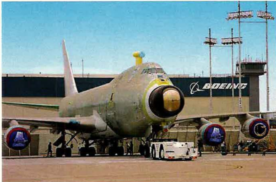
A large ball turret on the nose of the Airborne Laser will house the system optics. The full-up laser will be installed in the airplane in early 2004. Test shots against a Scud-type target are scheduled for summer 2004.
