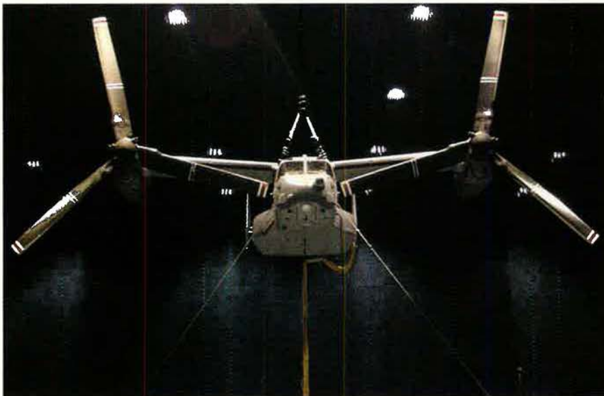
Hanging Around. A CV-22 is suspended in the Benfield Anechoic Facility at Edwards AFB, Calif., where it is undergoing tests of its integrated radio frequency countermeasures system.
