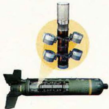
CBU-97 Sensor Fuzed Weapon with BLU-108 Submunitions
