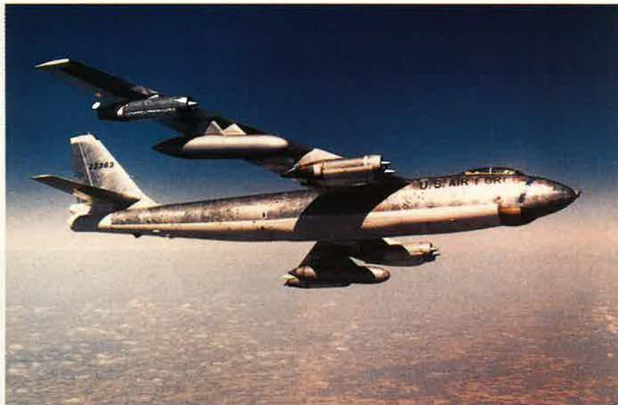
The medium-range B-47—the world's first swept-wing bomber—was developed about the same time as the long-range B-52. The design of the six-engine B-47 was so advanced that some called it futuristic.
