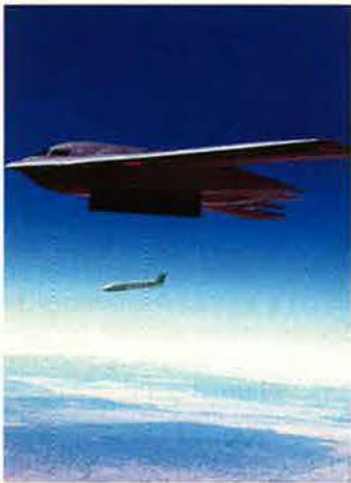
About the cover: A B-2 releases a Joint Air-to-Surface Standoff Missile on a test mission. See "Long Arm of the Air Force," p. 28.
