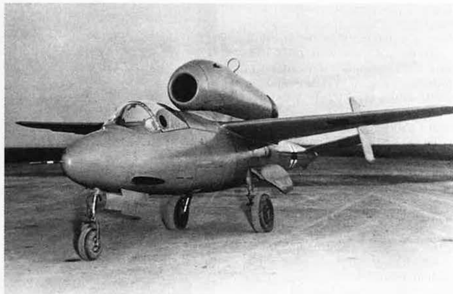
Late in the war, Germany grew desperate to turn the tide against the Allies. One proposal was the He-162 Salamander, a flimsy lightweight jet aircraft built partially out of plywood and intended to be expendable.
