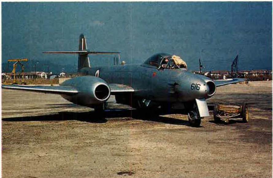
The Whittle engine was installed on the Gloster Meteor, the first Royal Air Force jet aircraft. Sixteen Meteors were delivered to RAF late in World War II. The first saw combat in August 1944.
