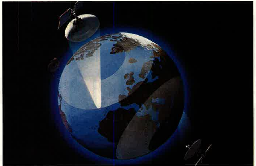
Undecided is whether SBR will be a constellation in low or medium Earth orbit or a combination of the two. Higher satellites provide greater coverage and can be fewer in number; lower satellites use less power and can be smaller.
