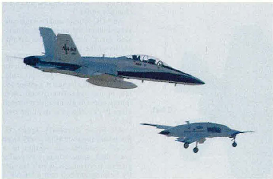
Gear was not retracted on the first flight, which is typical for a prototype. In combat, UCAVs may fly formation with manned aircraft, peeling off to strike pop-up air defense threats, or on their own, flying pre-emptive SEAD.
