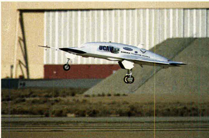
The UCAV flares for landing, after a 14-minute first flight. Handling qualities were judged to be good, and the no-tail airplane was stable throughout the flight. Testing will focus on mission, rather than violent maneuvering.
