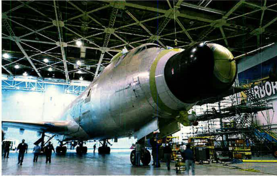
The first Airborne Laser aircraft, here at the Boeing facility in Wichita, Kan., is ready for airworthiness testing to see if it still flies like a 767 despite structural changes. (See "Laser-Less ABL Ready for Flight," below.)
