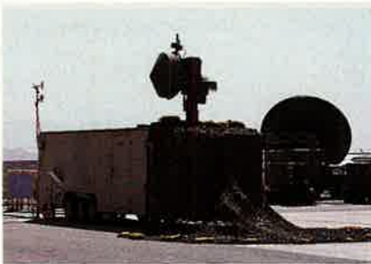
The aircrew and sensor crews both operate from the Ground Control Station. The GCS is housed in what looks like a camouflaged shipping container. The system's 20-foot-diameter satellite dish connects the GCS and the UAV when it is beyond line-of-sight range and also disseminates intelligence.
