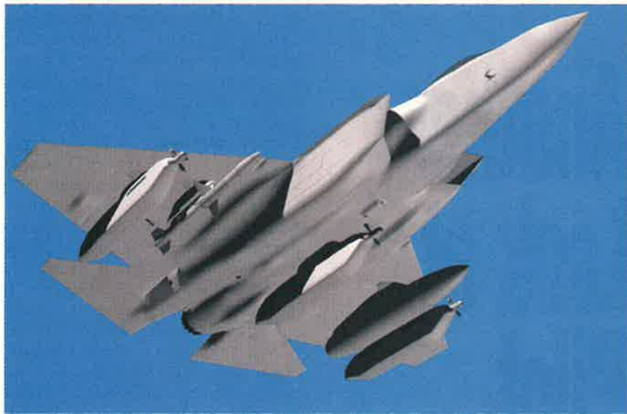
An electronic attack version of the JSF might make sense as the next jammer platform, but it doesn't arrive until 2010, leaving a gap in coverage. One JSF option (top) is for a "clean" version with EW gear carried internally. Another idea (here) would use external pods already in the works for the EA-6B.
