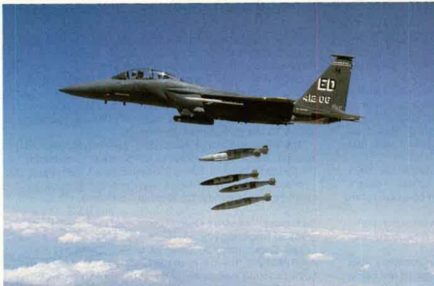
Lt. Col. Troy Fontaine, test pilot, and Maj. Kevin Steffenson, weapons system officer, launch five Joint Direct Attack Munitions from an F-15E over a California test range and, using GPS coordinates, successfully hit five separate targets.
