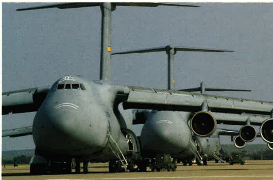
The C-5 remains a uniquely capable large airlifter, but poor reliability has made it a drag on the mobility fleet. An upgrade and re-engining program will be tested in time to decide whether to refurbish old Galaxys or simply buy more C-17s.
