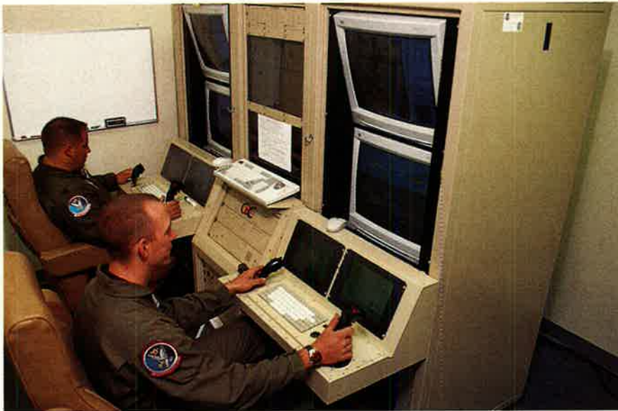
The aircrew and sensor crews both operate from the Ground Control Station. The GCS is housed in what looks like a camouflaged shipping container. The system's 20-foot-diameter satellite dish connects the GCS and the UAV when it is beyond line-of-sight range and also disseminates intelligence.
