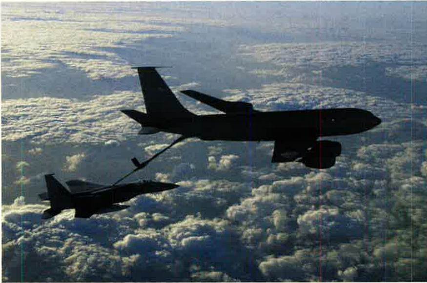
The war in Afghanistan would not have been possible without a massive tanker effort. The 40-year-old KC-135s are afflicted with corrosion and other problems, and USAF is eyeing a lease or buy of new militarized 767s as replacements.
