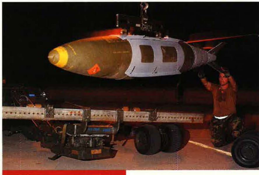
Makeover. A low-cost tail kit turns a standard 2,000-pound iron bomb into an all-weather, day-or-night Joint Direct Attack Munition.
