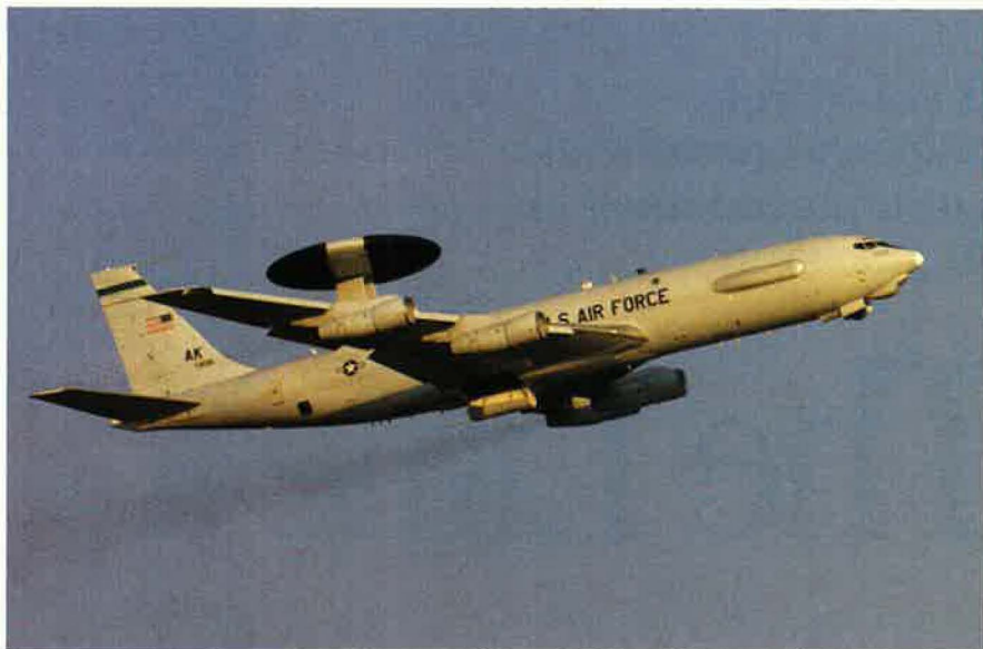
USAF has enhanced the capabilities of E-3s over the years. The E-3C featured circa 1984 console and radar improvements. With Extend Sentry, begun 10 years later, the service will upgrade everything from software to the airframe.
