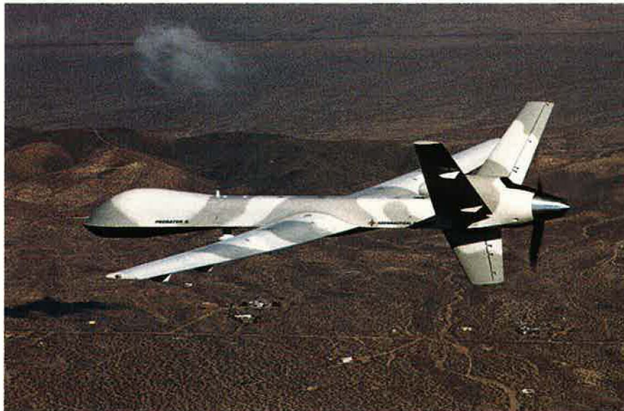
The Predator B, shown here, is a larger version of the RQ-1 above. It is nine feet longer, has a wing span 18 feet wider, and is nearly twice the weight of the original. It can reach speeds of nearly 250 mph and altitude of 45,000 feet.
