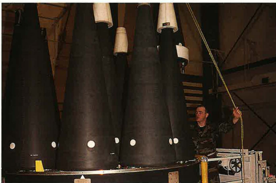
Fewer Warheads. The Bush plan calls for cutting deployed warheads by two-thirds, at least. Here, a USAF maintainer fits the last of 10 re-entry vehicles atop an LG-118A Peacekeeper ICBM.
