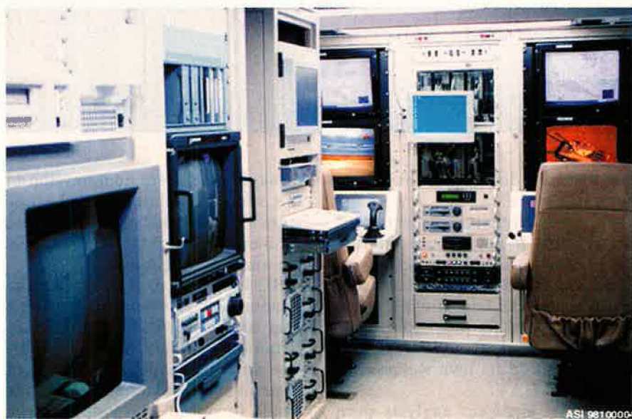
The Predator Ground Control Station is the largest component and is designed to roll onto a C-130. The GCS crew is an air vehicle operator—the "pilot"—and three sensor operators.
