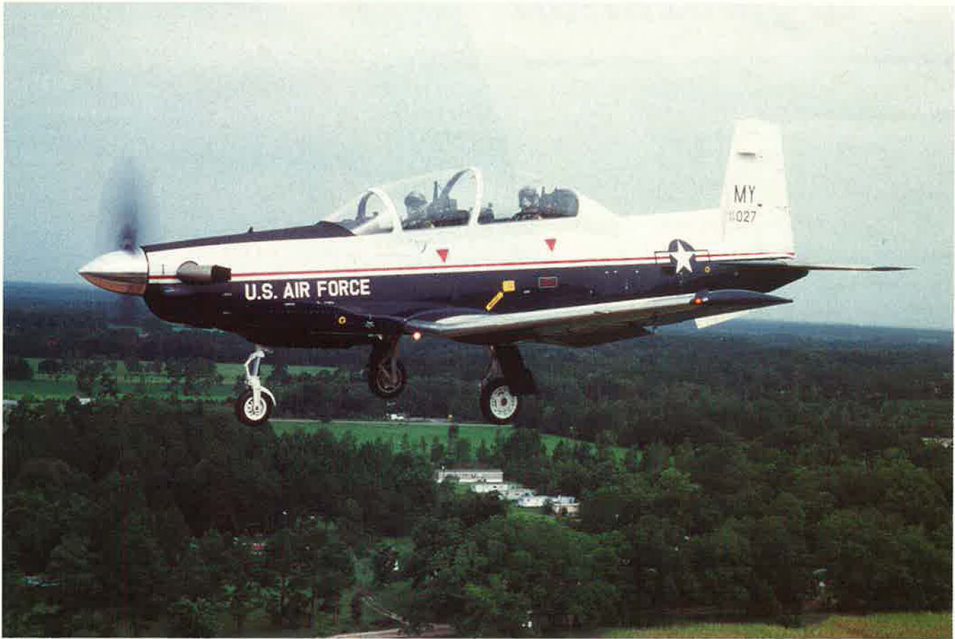
The trainer's tricycle-type landing gear is down and locked as the T-6A above makes its final approach to Moody.
