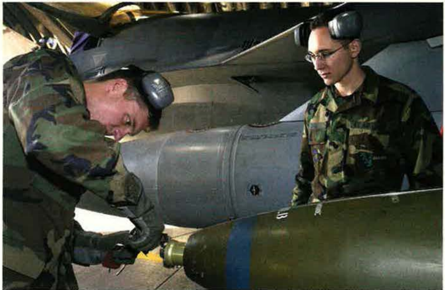
A1C Jerry Pierson, 555th Fighter Squadron, Aviano AB, Italy, tightens the arming wire on a bomb as SrA. Patrick Dull, a load standardization instructor with Aviano's 31st Operations Group, watches closely.
