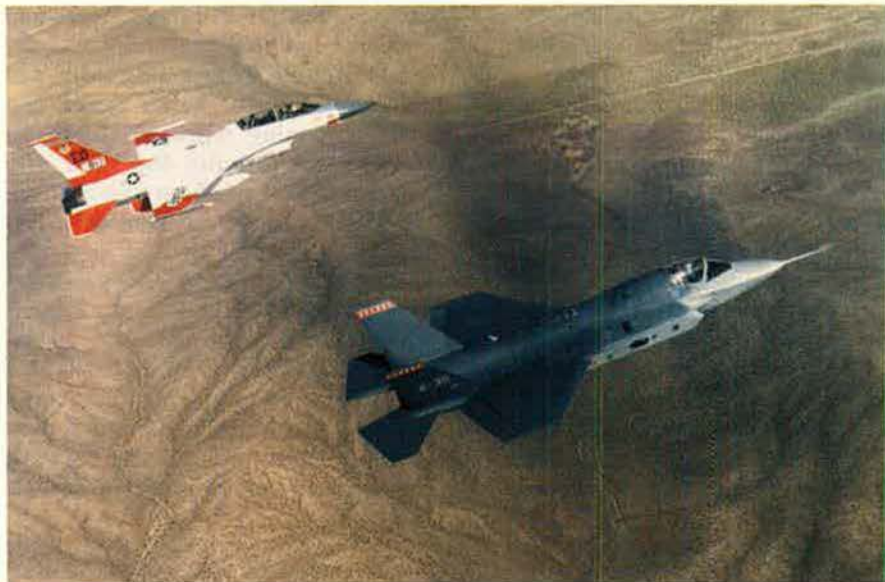
The new fighter's outline will be only slightly larger than the F-16 but with a much deeper fuselage for stealthy internal weapons and fuel carriage. When stealth is less of an issue, external stores can be carried on wing hardpoints.
