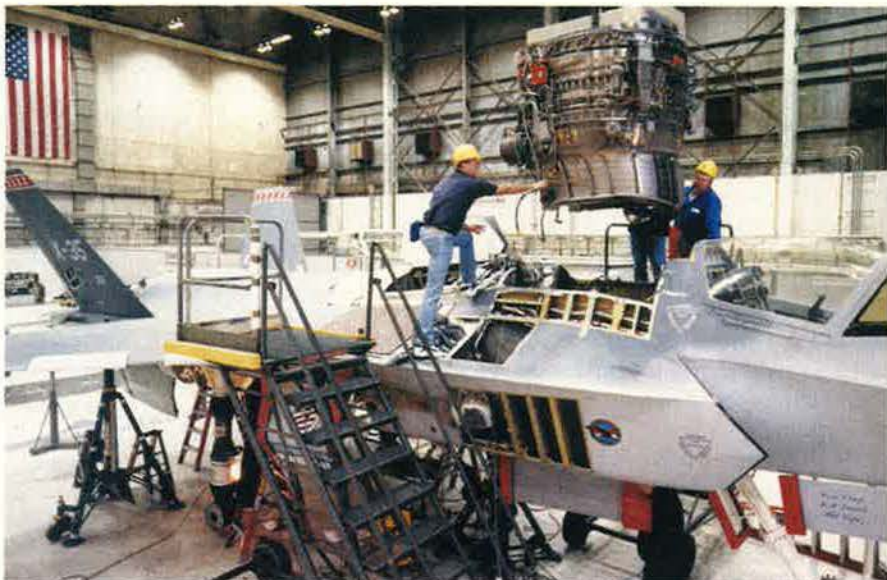
On the Marine Corps/UK model, the lift fan is installed behind the cockpit to enable vertical takeoff and landing. In the Air Force and Navy versions, this space is used for fuel, adding hundreds of miles of range.
