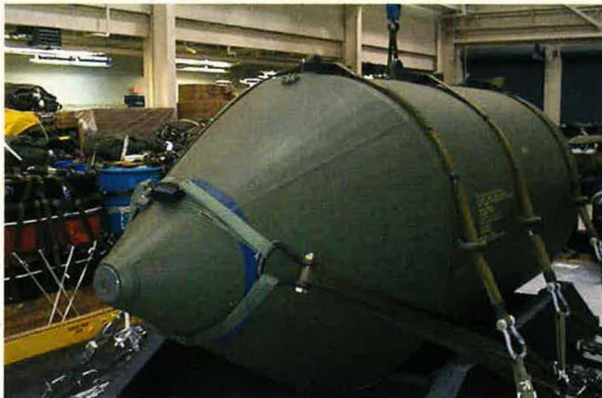
Used in Commando Vault missions in Vietnam to clear landing areas, the BLU-82 15,000-pound free-fall bomb, known as the "Daisy Cutter," has proved effective against Taliban and al Qaeda forces. The bomb is so huge, it's pushed out the back of special operations C-130s and drops by parachute. It's being used in Afghanistan largely for its intimidation effect. As Air Force Gen. Richard Myers, JCS Chairman, told reporters who asked about results: "Dead al Qaeda."
