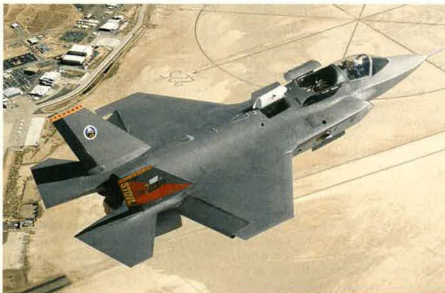
Both teams agreed that Lockheed Martin's Short Takeoff and Vertical Landing concept was one of the clinching factors. A "lift fan" behind the cockpit, powered by a shaft from the engine, helps loft the airplane while adding payload margin.
