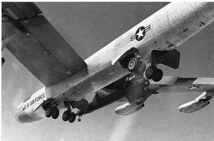
Only three A model B-52s were produced. One—designated NB-52A—served as the mother ship for the X-15 research aircraft and other test vehicles until 1968. After that a B model—NB-52B—took over.
