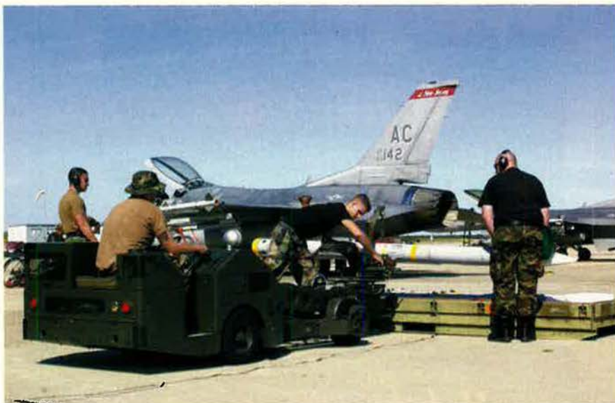
A New Jersey ANG weapons load crew raises an AIM-120A missile to transport it to an F-16C going out on stateside Combat Air Patrol. Since Sept. 11, the Guard has maintained aircraft aloft over various cities and on "strip alert."
