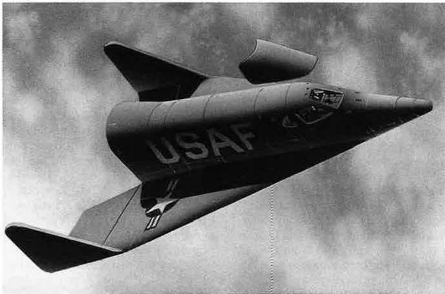
The quest for hypersonics and reusable spaceflight led in 1957 to the Dyna-Soar X-20. It was designed to be a manned orbital craft and did contribute to the space shuttle program but was canceled in 1963. (Artist's concept)
