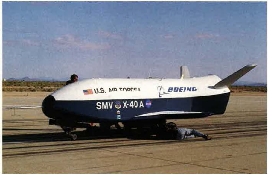
The second free flight of X-40A, an 85 percent scale version of the proposed X-37, took place earlier this year at Edwards. The unmanned X-37 was to be used as a test bed for some Space Maneuvering Vehicle concepts.
