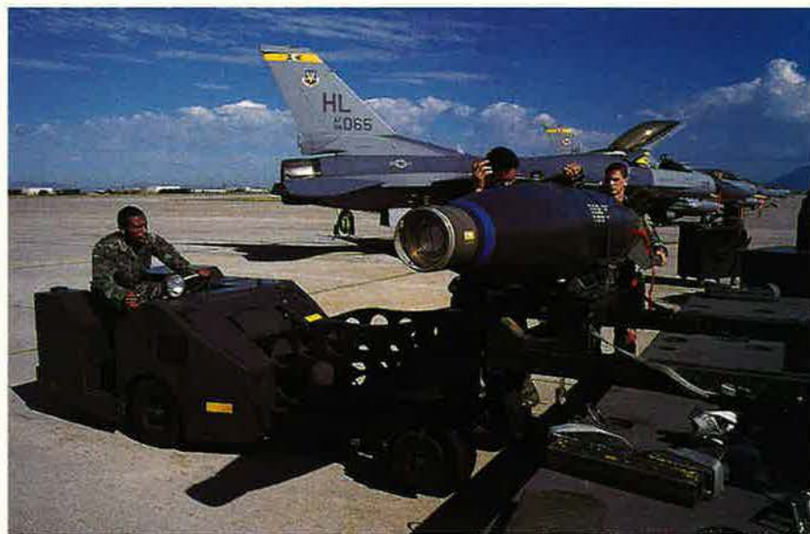
In Allied Force, many of the precision munitions, like the laser-guided bomb here, required the pilot to see a target to guide the bomb. That was no problem for fixed targets, but as the targets changed, the 15,000-foot rule was relaxed.
