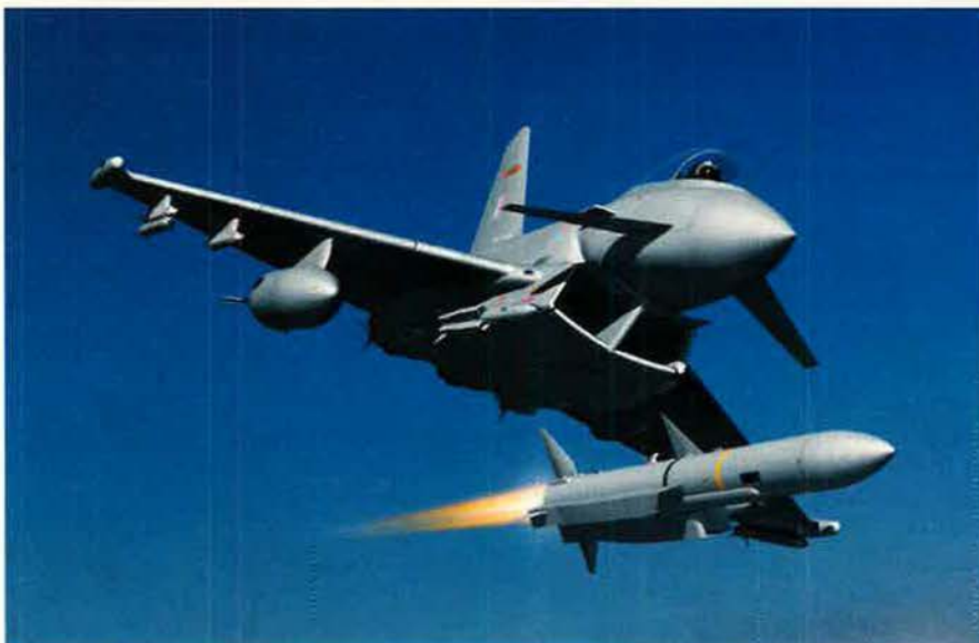
New, superfast, and extremely agile missiles pose an increased threat. The already potent Typhoon will give up its AMRAAMs for the Meteor, a ramjet-powered, long-range missile with high speed and resistance to countermeasures.
