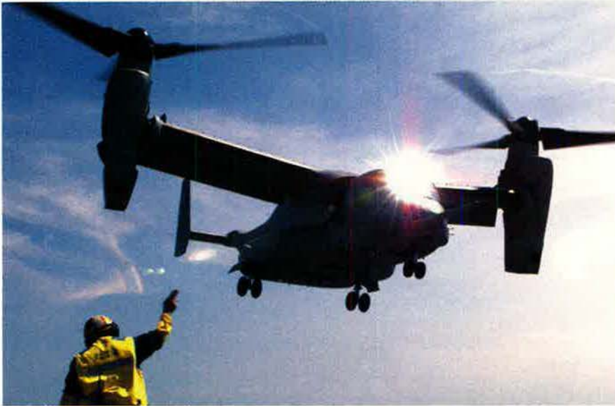
An MV-22B Osprey prepares to land on USS Saipan during testing. According to Marine officials, Osprey testing was based on schedule, rather than performance—a contributing factor in one, if not both, of the multifatality crashes last year.
