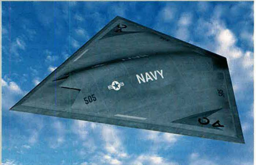
Physics, not aesthetics, drive stealth design, and the math says the shape with the smallest radar return is a diamond. Northrop’s Pegasus UCAV is aimed at a Navy contract for a carrier-based everyday scouting and attack robot.
