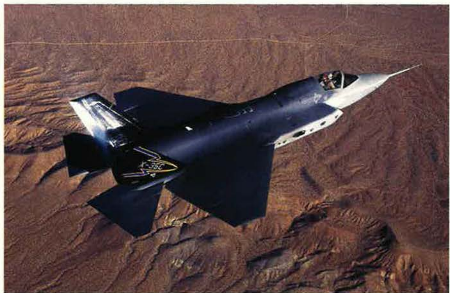
The X-32 and X-35 have racked up the smoothest-ever flight test program of X-planes, thanks to exhaustive simulation beforehand. Lockheed Martin's X-35, shown here, closely matches the company's proposed JSF design.
