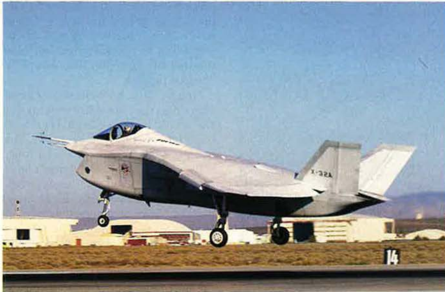
Boeing's tailless X-32 design has been superceded by the company's final JSF proposal, which has a more conventional layout. The JSF X-planes demonstrate design, flight, and manufacturing concepts and aren't meant to be prototypes.
