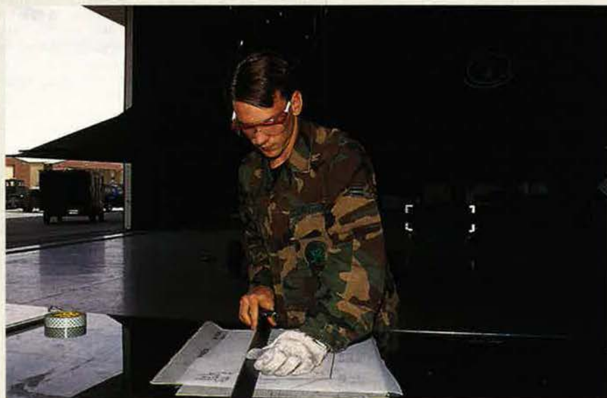
Known as "Martians" (shorthand for Materials Repair Specialist), F-117 technicians for years applied Radar Absorbent Materials in a fashion more akin to art class than metal shop. Here, A1C Kenneth Sheppa trims out a replacement piece.
