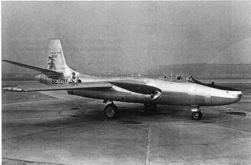
This RB-45C, a special version of the B-45 Tornado bomber, had five camera stations for its charting, mapping, and photoreconnaissance missions, which were carried out at high and low altitudes, day and night.
