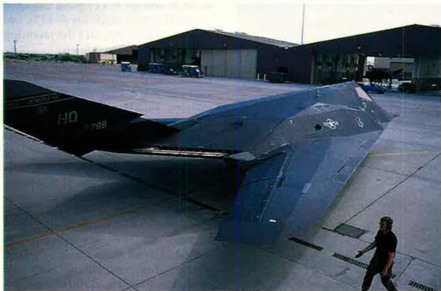
The “platypus” is the colorful name coined to describe the F-117’s unique exhaust. It hides the aircraft from infrared sensors by dispersing the exhaust heat over a wide area, mixing it with cool air and shielding it from ground view.
