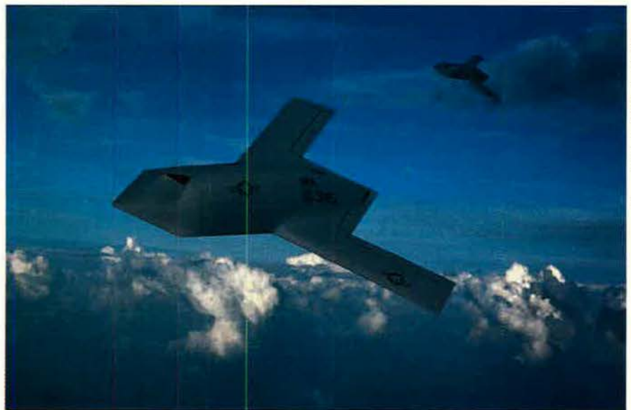
Hazardous Duty. UCAVs could be used for missions of extreme danger, such as attacks on air defense sites. Boeing’s X-45A UCAV (in artist’s depiction) rolled out last year.
