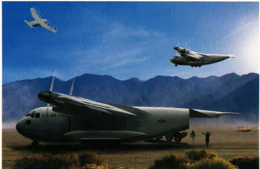
Vision Lift. One mobility idea is the Advanced Tactical Transport, a short-takeoff-and-landing aircraft that would eventually replace the C-130 for combat deliveries to austere airfields.
