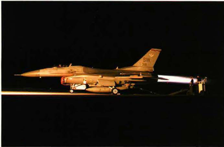
An F-16CJ runs in full afterburner during a nighttime engine test at Shaw AFB, S.C. SrA. James Kennedy controls the test from the cockpit. At the rear of the aircraft, A1C Justin Cox (left) monitors operations, while SSgt. Bryan Gallo stands by with fire extinguishing equipment.
