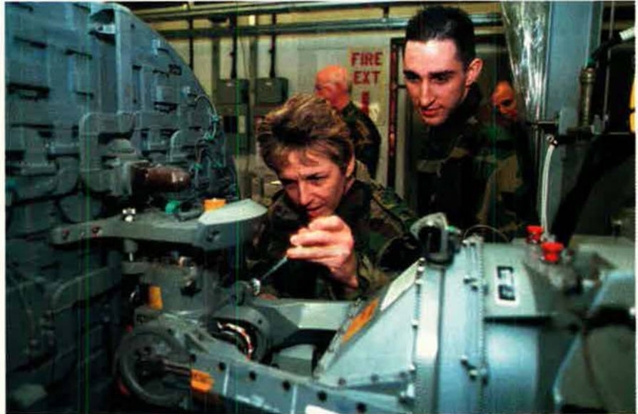
At RAF Lakenheath, UK, Brig. Gen. Terry Gabreski, USAF director of maintenance, performs an antenna boresight alignment as SrA. Greg Fedorick, from the 48th Component Repair Squadron's Avionics Flight, observes.
