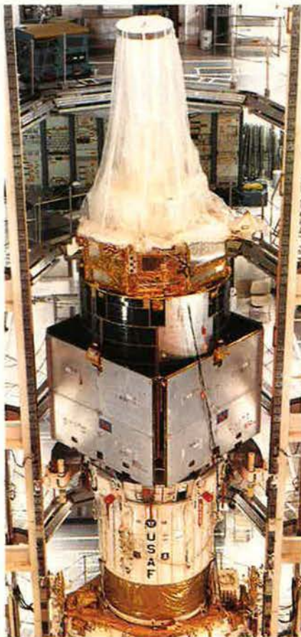
Defense Support Program satellite atop an Inertial upper Stage prior to launch. (NASA photo)
