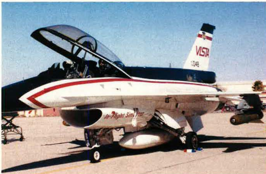
USAF Test Pilot School staff at Edwards AFB, Calif., recently flew the F-16 Variable Stability In-Flight Simulator Test Aircraft with two Maverick training missiles. The flights evaluated the ability of the VISTA to carry Mavericks to provide students with training in the differences between using visible and infrared sensors for acquiring and attacking ground targets.
