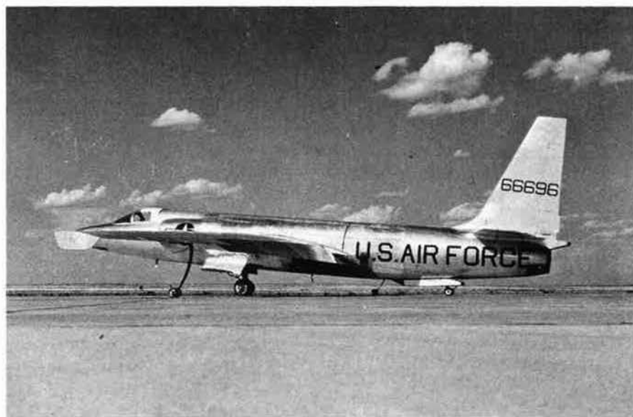
Above is a USAF U-2A. The Navy gave several U-2As stronger landing gear, an arresting hook, and spoilers. Designated U-2Gs, they were prepared for carrier operations in an effort to extend the range of US intelligence gathering.
