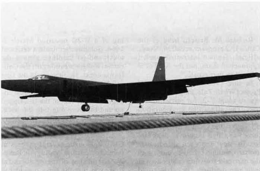
A U-2R undergoes carrier qualifications on USS America in November 1969. By this time, the spyplane was 40 percent larger than earlier versions, but its wings folded up and it required little special handling on the carrier.
