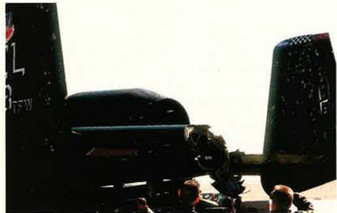
This close-up view of the tail section of a 23rd TFW A-10A aircraft from England AFB, La., shows the damage it sustained when an SA-16 missile exploded near it during Desert Storm.
