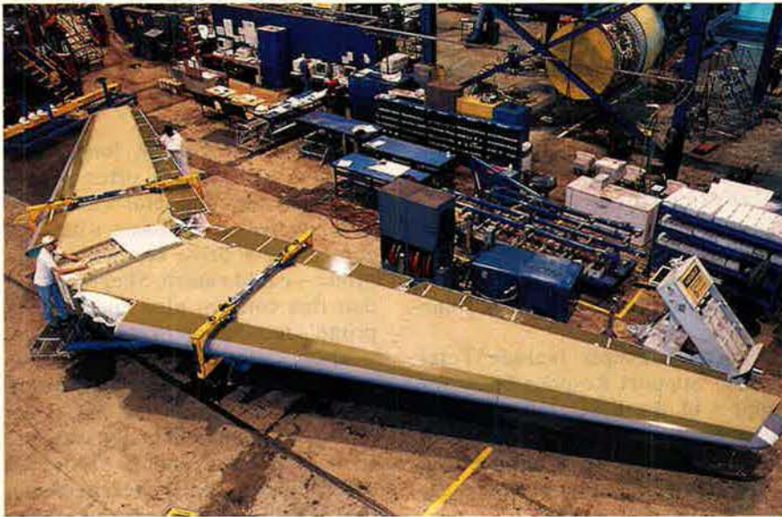
The first C-17 composite horizontal stabilizer is readied at Northrop Grumman. Ogden ALC's director said a viable depot must introduce new workloads, such as C-17 landing gear, to its workforce to maintain core repair capabilities.
