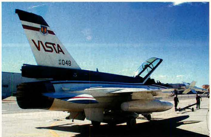
The NF-16D Variable-Stability In-Flight Simulator, Test Aircraft (above) recently arrived at the US Air Force Test Pilot School at Edwards AFB. The VISTA trainer can simulate fighters such as the F-15 and the Navy F-14 in flight and gives students an opportunity to learn how to test future integrated cockpits.
