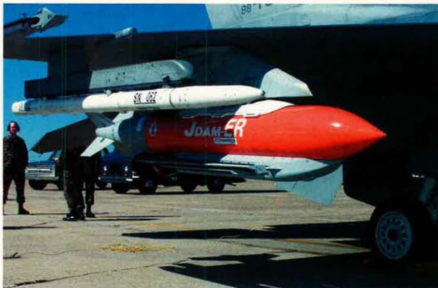
The Joint Direct Attack Munition-Extended Range is shown on an F-16 before a cross-range flight test at White Sands Missile Range, N.M. The JDAM-ER uses a strap-on wing device called a Diamond Back—a low-cost, high-performance wing kit that increases the JDAM's range and allows attack on multiple, widely separated targets from a single release point.
