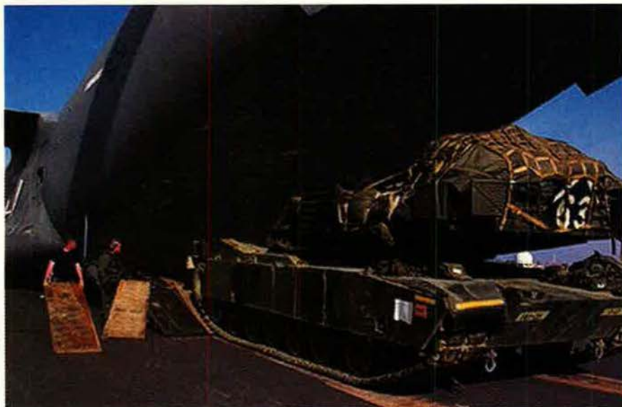
The beast in the belly. The C-17 (shown here) is the only USAF cargo aircraft that can both carry an Abrams and land on an unimproved strip. The airlifter can haul only one big tank per trip, however.
