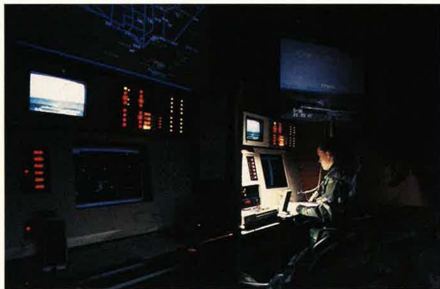
The integrated and instrumented range complex at Nellis affords control from the ground. The Red Flag Measurement and Debriefing System, TV ordnance scoring, and threat video are part of a lessons-learned replay afterward.
