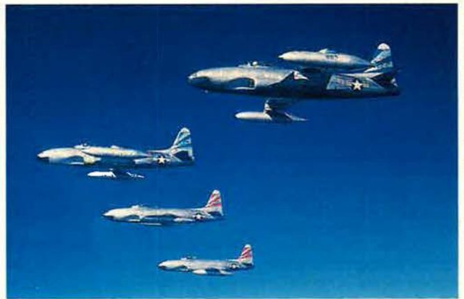
Four F-80s head into battle. USAF's first operational jet fighter, the Shooting Star flew extensively in the Korean War in the ground attack role.
