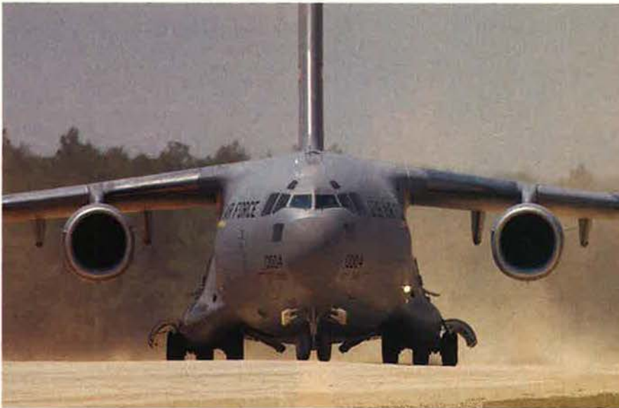
A C-17 from Altus AFB, Okla., performs an assault landing on a dirt landing strip. Aircraft in this Rodeo event aimed for a smooth, consistent approach to a specific point 250 feet into the touchdown zone and received points for proper speed, smooth approach, and landing without bouncing.
