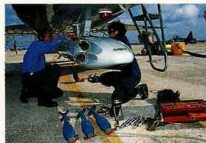
The AT-38 is only slightly different from the T-38 the students flew during SUPT. It has a notional gunsight and a centerline hardpoint that the ground crew below is using to attach an SUU-20 bomb dispenser. The weapons pod contains as many as six small blue practice bombs that produce white smoke on contact with the ground.
