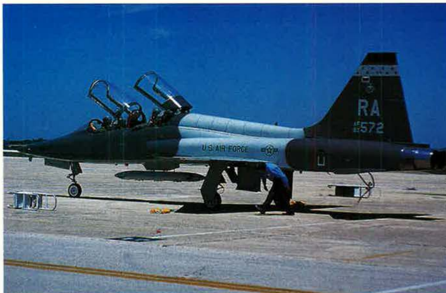
The AT-38 is only slightly different from the T-38 the students flew during SUPT. It has a notional gunsight and a centerline hardpoint that the ground crew below is using to attach an SUU-20 bomb dispenser. The weapons pod contains as many as six small blue practice bombs that produce white smoke on contact with the ground.
