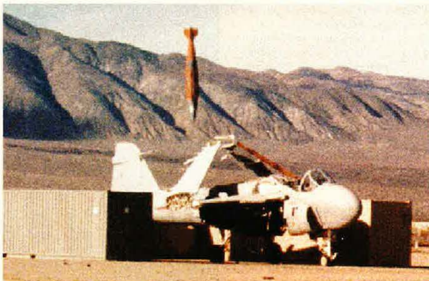
JDAM was the star performer of Allied Force and vindicated USAF's move to GPS-aided weapons. Seen here in a test against an A-6 carcass, JDAM is classed as a near-precision weapon but routinely hits within 40 feet of its target.
