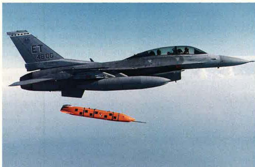
The next major advance in precision attack will come from JASSM, here being tested from an F-16D. The JASSM is stealthy, can fly hundreds of miles, and can strike hardened targets with high accuracy.
