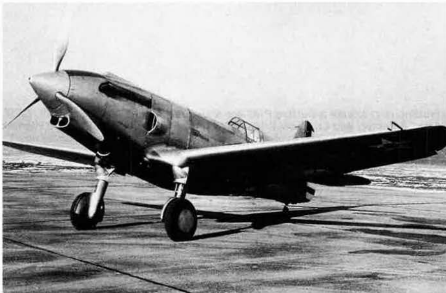
An unusually skillful pilot, Alison said if you could fly one airplane, you could fly them all. Among the lesser known aircraft he flew: a P-37 like this one, a variant of the radial engined P-36, designed around an Allison V-1710-11 engine.
