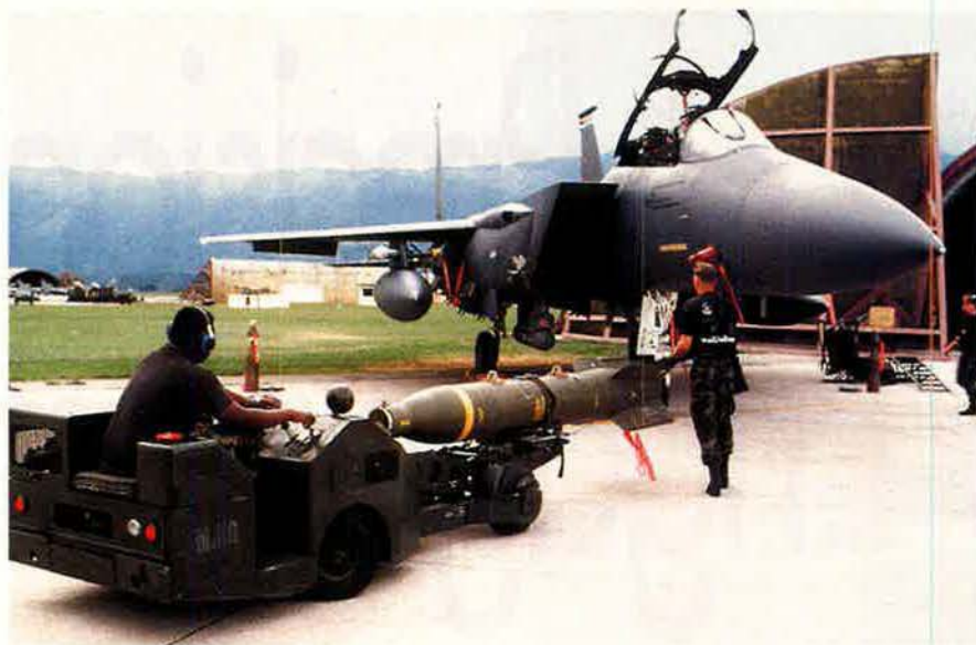
Use of precision weapons has expanded greatly since the 1991 Gulf War. Nearly all munitions used in NATO's Operation Deliberate Force in 1995 were PGMs. Here, an F-15E is loaded with a Laser-Guided Bomb at Aviano AB, Italy.
