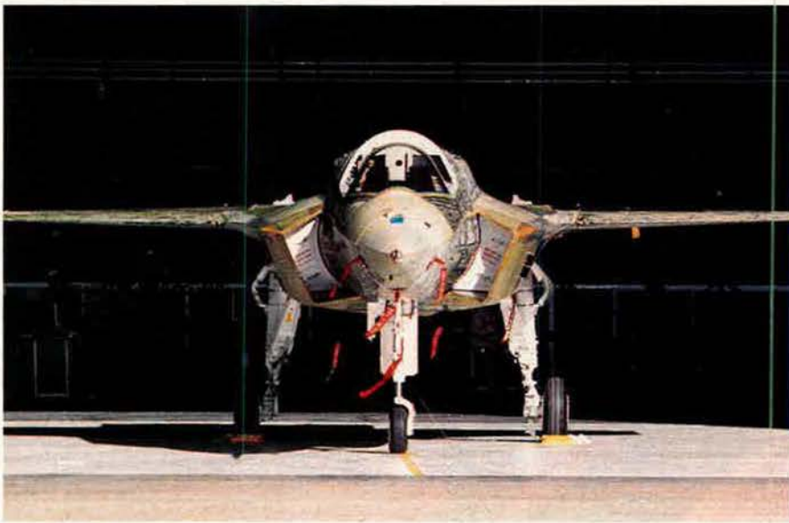
Lockheed Martin's Joint Strike Fighter concept demonstrator, the X-35A, had its first flight engine installed at the Lockheed Martin Skunk Works in Palmdale, Calif., on Dec 9. The X-35A's first flight is scheduled for spring.
