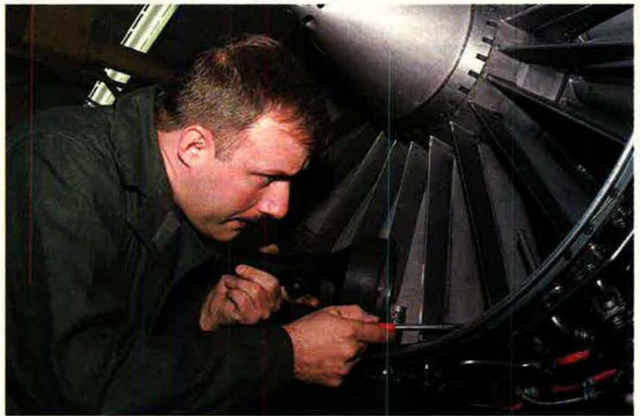
TSgt. Jim Strand inspects an F-16's F100-PW-220 engine for spots or cracks. Following a series of F-16 crashes, maintainers at Luke AFB, Ariz., worked with the contractor and San Antonio Air Logistics Center to develop a more comprehensive inspection, using improved cleaning procedures and an oil-based penetrant to find cracks that previously went undetected.
