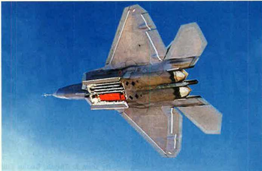
The F-22 can handle six AMRAAM missiles in its weapons bay. For ground attack, it can carry two 1,000-pound, satellite-guided JDAMs. Though chiefly a guarantor of air superiority, every F-22 will also have a formidable attack capability.
