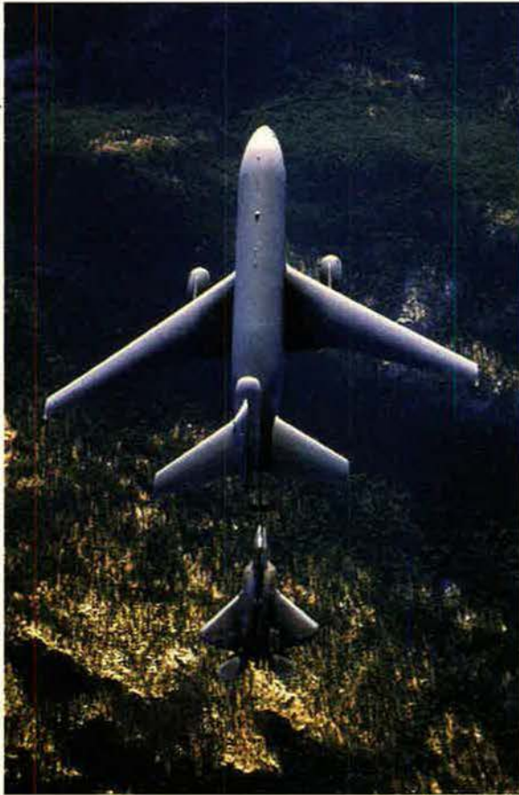
An F-22 connects with a KC-10 from Travis AFB, Calif., during a series of tests that determined the Raptor's compatibility with the tanker. The five days of testing in November helped identify the F-22's minimum and maximum allowable airspeeds, altitude, and tolerance for boom movement during refueling. In the testing period, KC-10s transferred 35,000 pounds of fuel.
