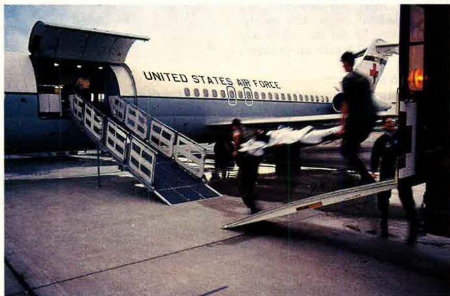
Long-distance air evacuation from Vietnam to the Philippines, Japan, and the US spurred USAF to acquire specially built C-9 Nightingale hospital aircraft. The C-9 can carry 40 litter patients with five medical personnel.
