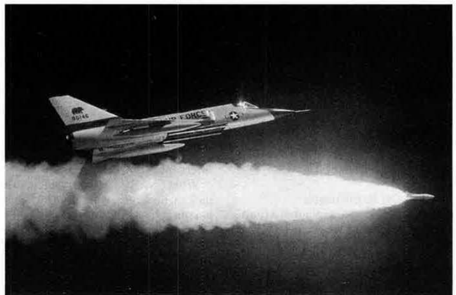
An F-106 launches an ATR-2A (the training version of the AIR-2A Genie rocket). Operating with the SAGE system, the Delta Dart could be flown automatically from wheels up to flareout before touchdown.
