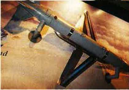
Above, Alenia Marconi featured a low-cost wing kit that could be used on a number of bombs. Company officials said the kit is designed to give longer range and greater maneuverability to weapon systems such as the joint direct attack munition and the wind-corrected munitions dispenser.
