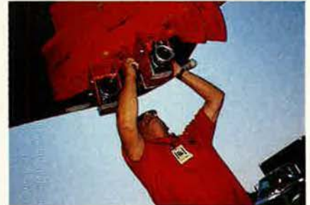
A1C Richard Kleen (left) and SSgt. David Currie carefully position the weapon on an F-15E for the drop test. Everything must be right to ensure that a test subject is not accidentally lost. Below, a tech rep positions cameras that will record every instant, at every angle, of the release.
