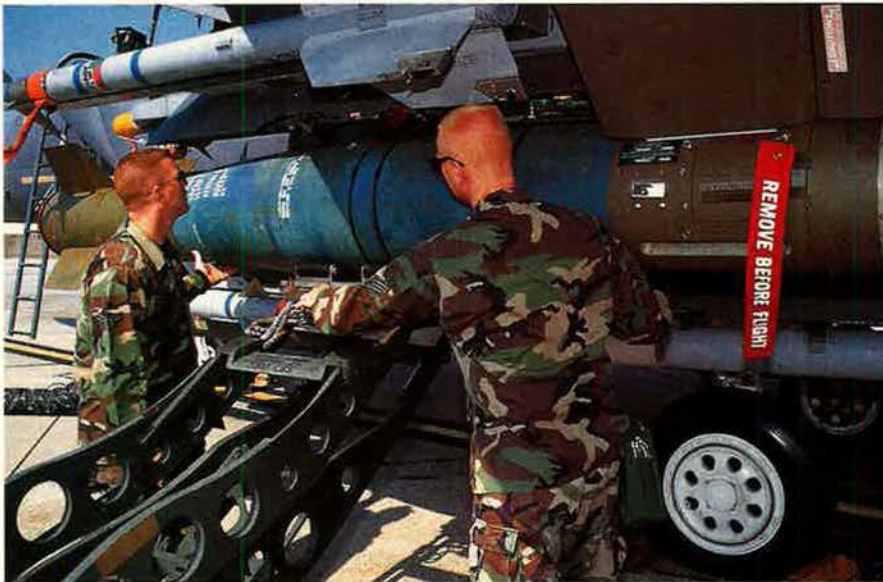
A1C Richard Kleen (left) and SSgt. David Currie carefully position the weapon on an F-15E for the drop test. Everything must be right to ensure that a test subject is not accidentally lost. Below, a tech rep positions cameras that will record every instant, at every angle, of the release.
