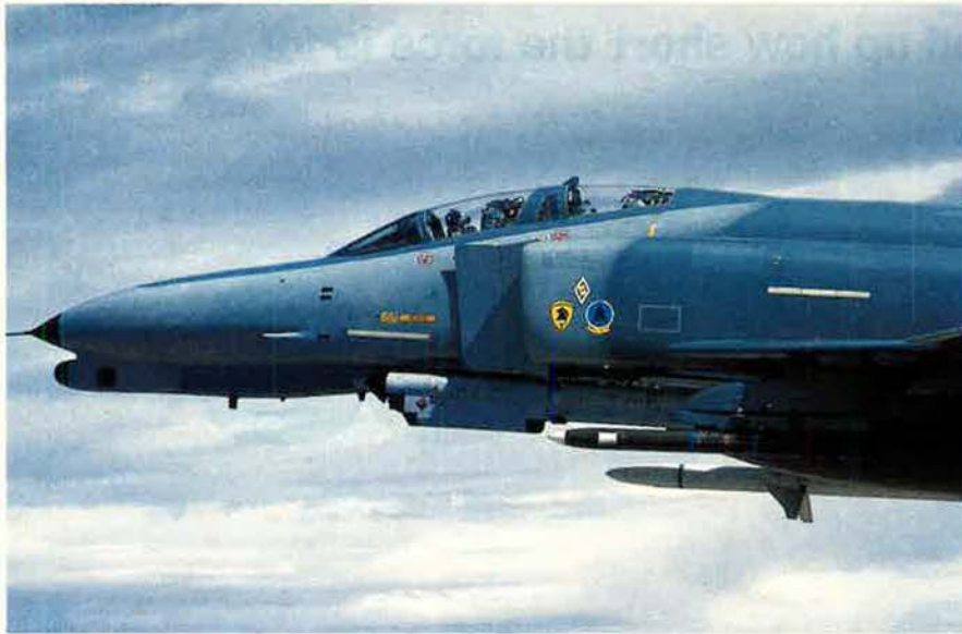
The F-4G was the king of SEAD from Vietnam to the Gulf. The backseater would interpret waveforms and sounds of enemy radars and select threats to attack in order of priority. The HARM Targeting System lacks the F-4G's range and precision, but it automates threat ranking for a solo pilot.
