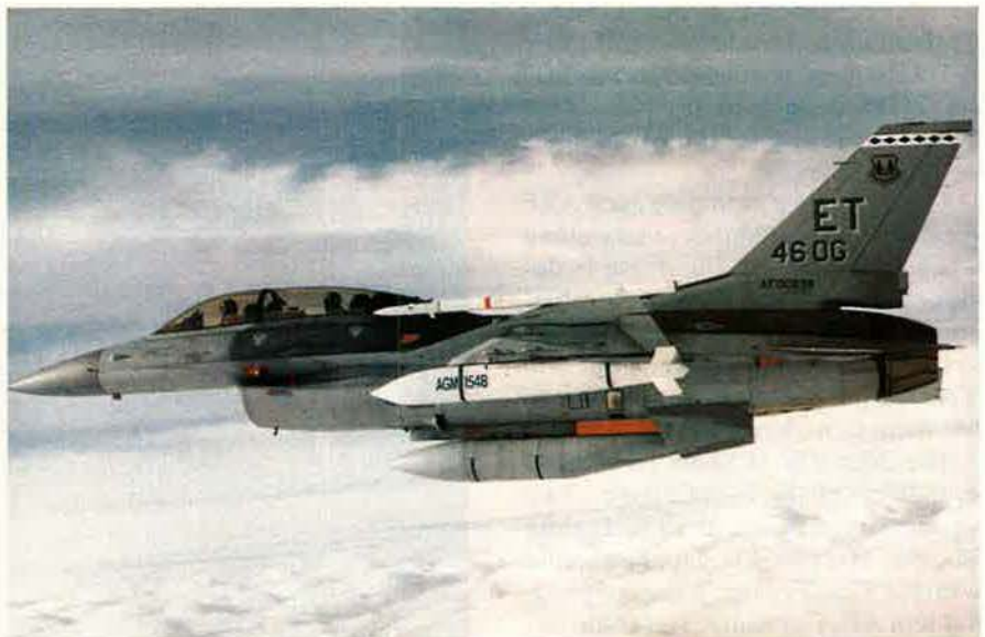
The joint standoff weapon, with high potential for defeating air defenses, is a new stealthy glide bomb with global positioning system accuracy. It can be released well away from SAMs—at a safe distance for airplane and pilot.
