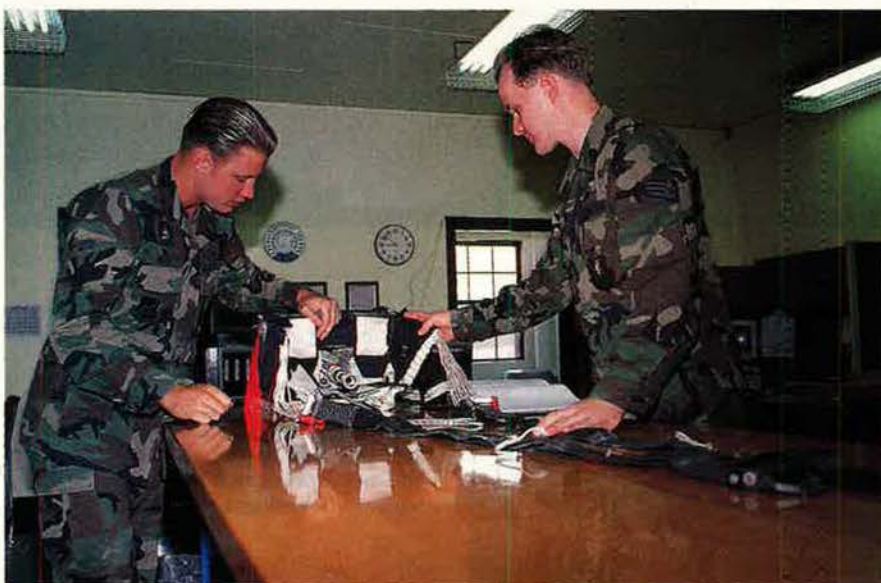
At left, A1C Scott A. Wcld and SSgt. Dale E. Ludwig inspect an ejection seat's parachute and harness system. Regular and detailed inspection is important to make certain this equipment works as expected. The specialists in the survival equipment shop perform detail work that may go unnoticed—until an aircrew finds itself in an emergency.
