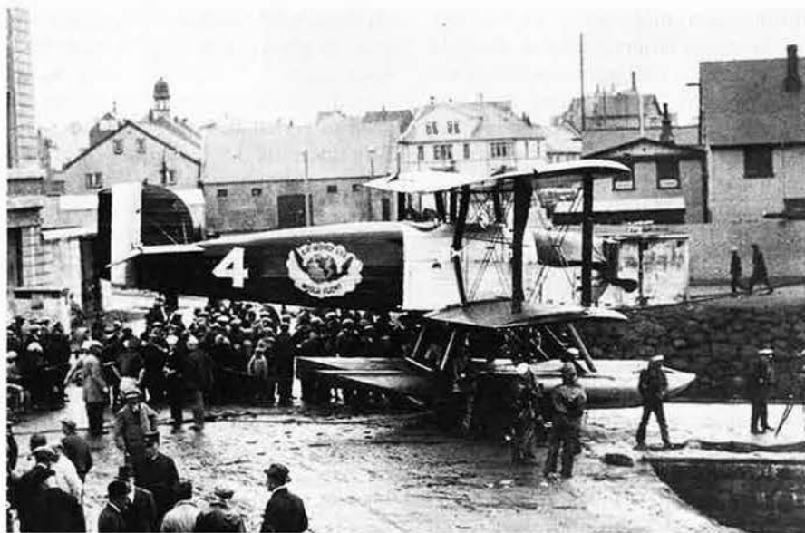
Enthusiastic crowds, like this one in Reykjavik, Iceland, greeted the aviation pioneers. Here, New Orleans is lifted from the water for an overhaul. It was still outfitted with pontoons which would be exchanged for wheels in Boston.
