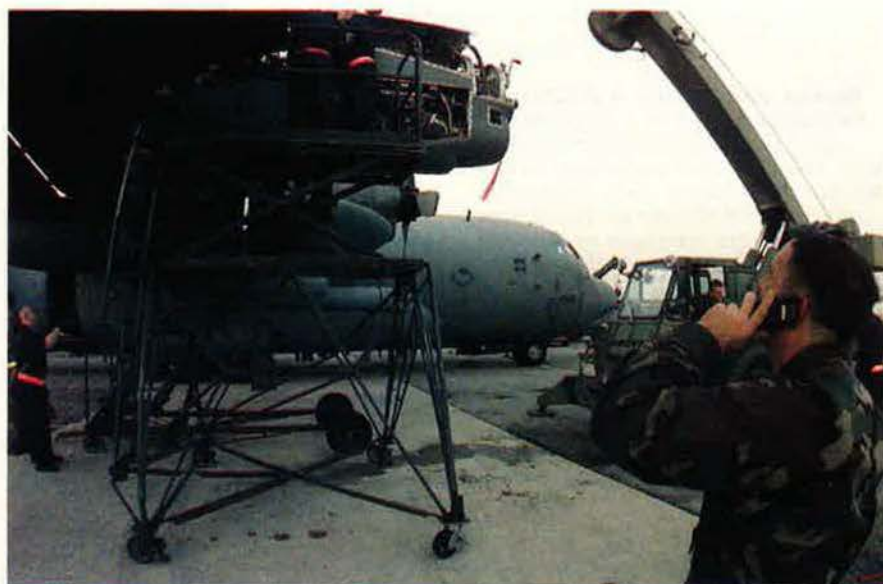
Fighting Trim. At Aviano, maintenance crews from the 43d Expeditionary Electronic Combat Squadron, located at Davis-Monthan AFB, Ariz., work on April 2 to replace an engine on their EC-130H Compass Call airplane. Below, SSgt. Paul Guyer, from the 510th FS, at Aviano, checks out his F-16 before he'll let the pilot fly it on a planned April 2 mission.
