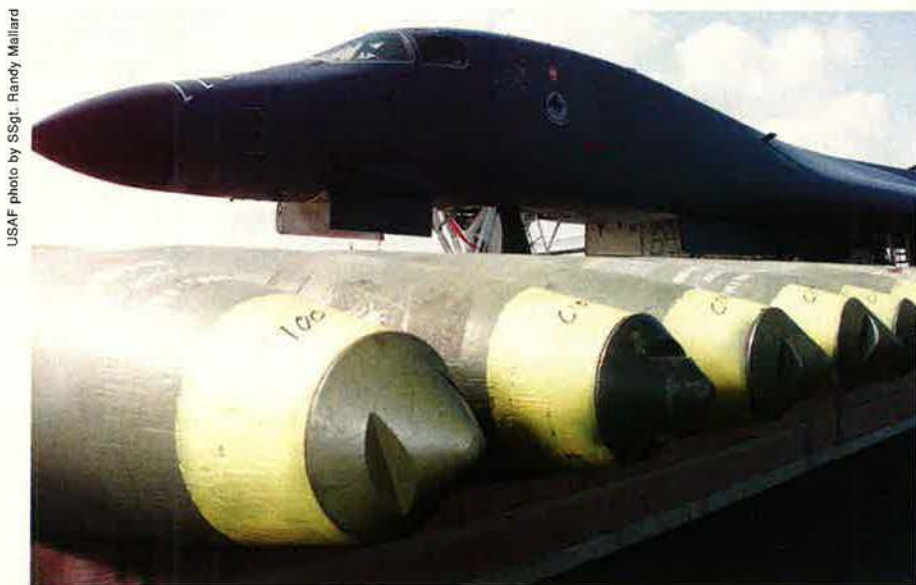
Today, B-1Bs carry dumb bombs like these Mk 82s. Soon, all bombers will have capability for precision weapons and USAF will be able to merge mass and precision in the same platforms.
