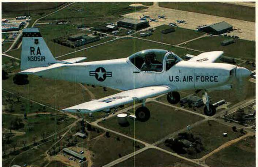
The T-3A had been used to screen candidates before they entered undergraduate pilot school, but USAF suspended Firefly operations in July 1997 after a series of accidents that have been linked to the engine's fuel supply system.
