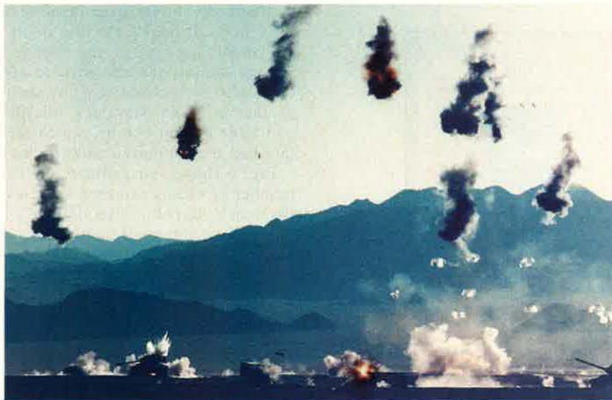
A single F-16 can carry four CBU-97 Sensor Fuzed Weapons and could be expected to engage around 30 armored vehicles and damage approximately half of them.
