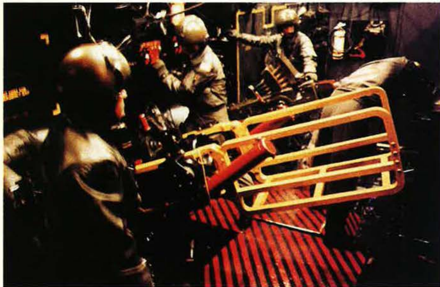
Pave Aegis upgrades added a 105 mm gun to the AC-130, making for less space in an already cramped gunner's station. The yellow safety cage protects crewmen from the gun's recoil. This gunship was photographed in the late 1980s.
