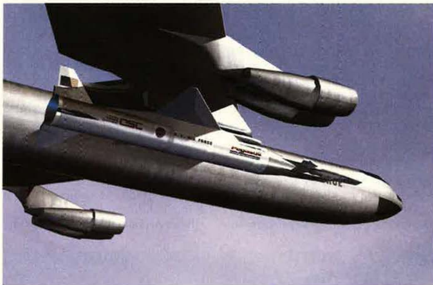
What comes around goes around. The very same B-52 that launched the X-15 will carry aloft the Pegasus/Hyper-X combination for three test flights, in 2000 and 2001. Pegasus is a proven launch capability, having put many small satellites into orbit.
