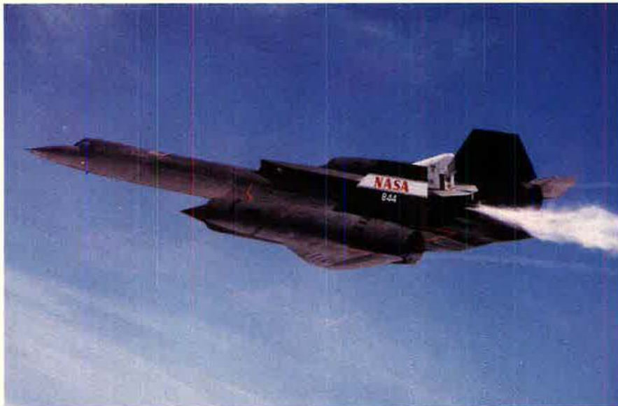
To test fast, you have to go fast. This Mach 3-plus SR-71 is carrying a linear aerospike engine on its spine for high-speed evaluations. In larger form, the aerospike will power the X-33 and possibly offer a much cheaper way to orbit.
