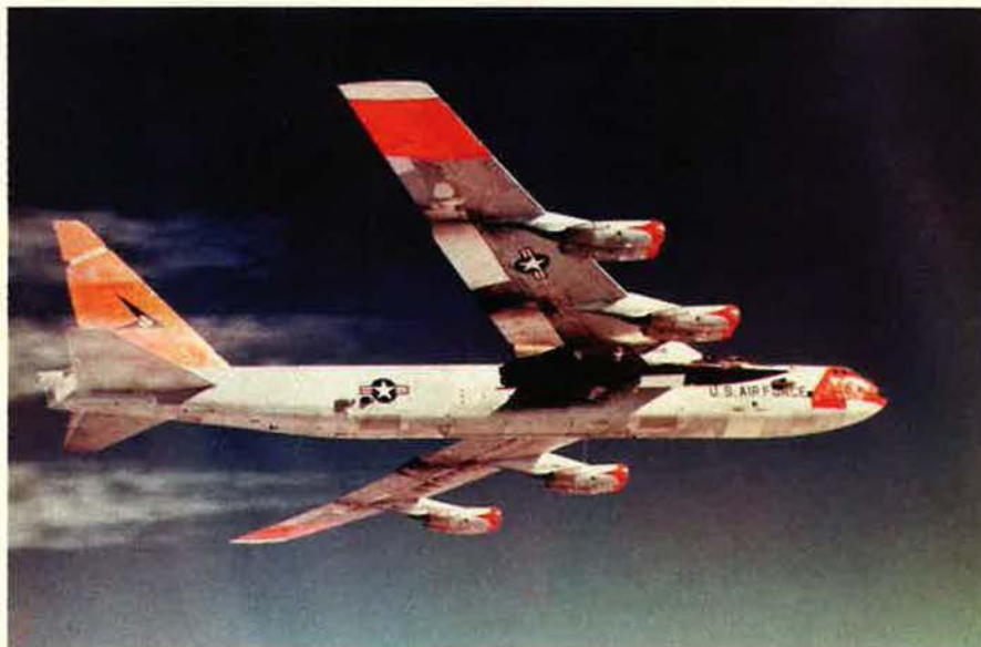
The celebrated X-15, shown here under the wing of its B-52 mother ship, reached Mach 6.7 and blazed a trail for the space shuttle. Hypersonic research is now aimed at reusable, more "operational" craft.
