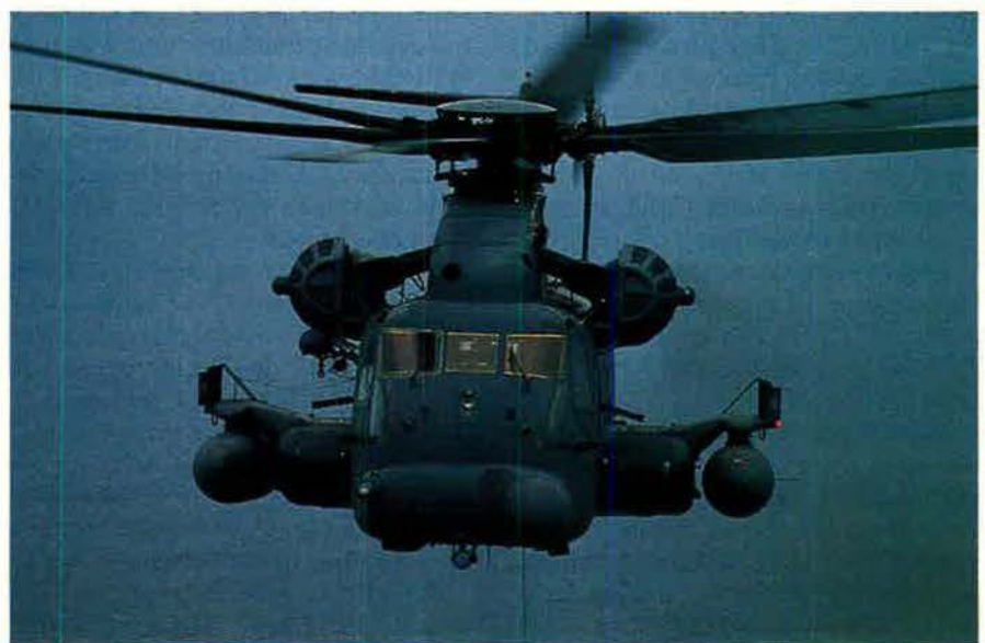
Looking like a Rube Goldberg special, the MH-53J Pave Low III has been heavily modified with strap-on fuel tanks, terrain-following radar, night vision equipment, and countermeasures. The CV-22 carries this gear internally.
