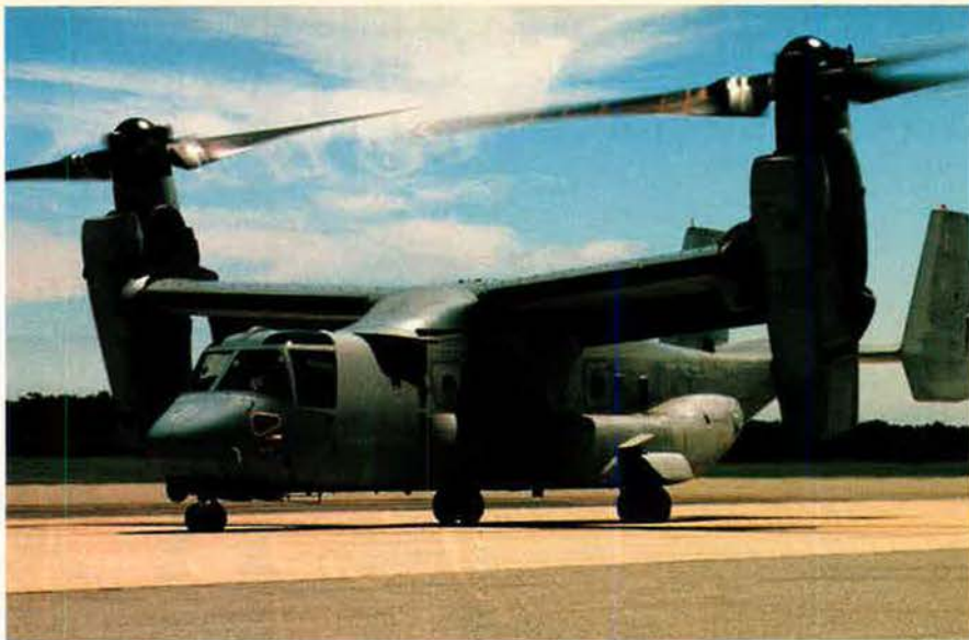
A V-22 in helicopter mode for takeoff. The Osprey is the first aircraft ever to combine vertical takeoff and landing with long range, high speed, and a big payload—just the ticket to give SOF units a quick, covert ride to the action.
