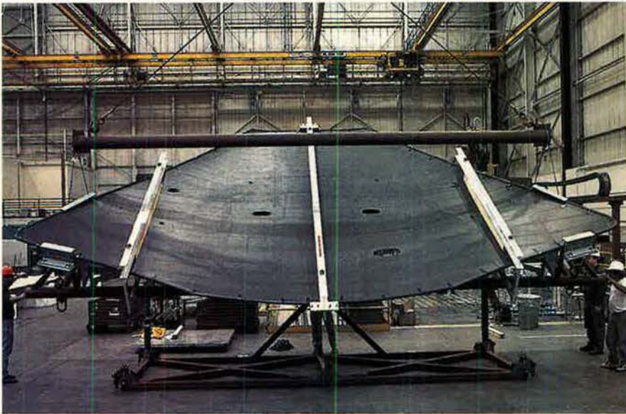
The Joint Strike Fighter X-32A concept demonstrator moved closer to completion as Boeing employees prepared the first composite wing skin for shipment to its final assembly plant in Palmdale, Calif., in November. Boeing is competing to build the JSF under a joint-service concept demonstration contract.
