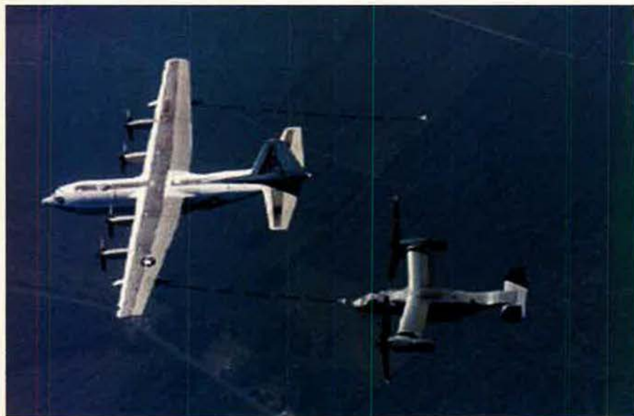
The Osprey is a big aircraft, at nearly half the size of a C-130. Its extended range will reduce the number of refuelings needed, permitting retirement not only of the MH-53 force it will replace but of some MC-130 tankers as well.
