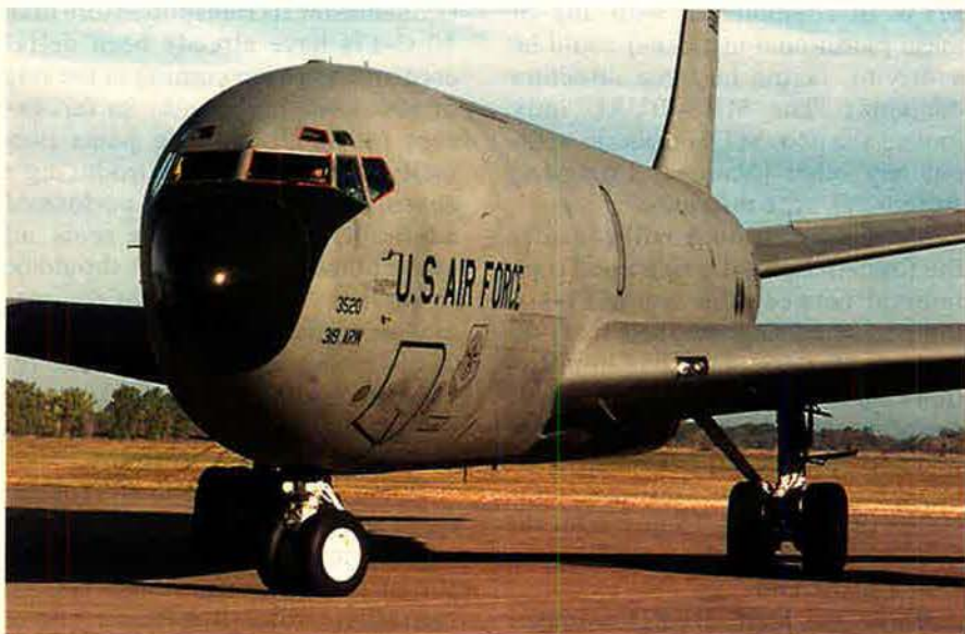
The first PACER CRAG KC-135 arrives at the 905th Air Refueling Squadron, Grand Forks AFB, N.D. An updated cockpit and radar, plus GPS and other navigation improvements, will make the tanker viable for decades more.
