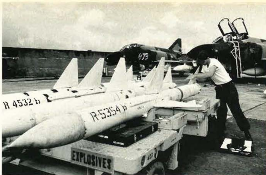
The F-4 carried four close-range AIM-9 Sidewinder heat-seeking missiles and four radar-guided AIM-7 Sparrows like those shown here. In the opening moments of Operation Bolo combat, Olds scored his first MiG-21 kill with an AIM-9.
