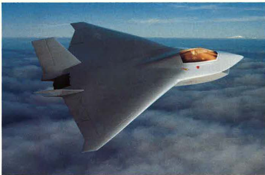
The JSF will reduce cost by limiting parts count. Almost the entire wing/upper fuselage of the Boeing design is a single piece of thermoplastic composite, the same for all variants. Commonality—avoiding unique parts—cuts unit cost.
