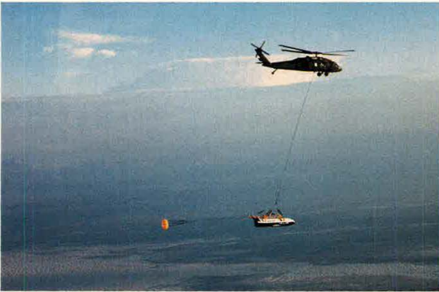
An Army helicopter on Aug. 11 prepares to drop a 90-percent scale version of USAF's Space Maneuver Vehicle. The SMV is a reusable, unmanned vehicle intended for potential use for reconnaissance, surveillance, or communications; stated Air Force Research Laboratory officials.
