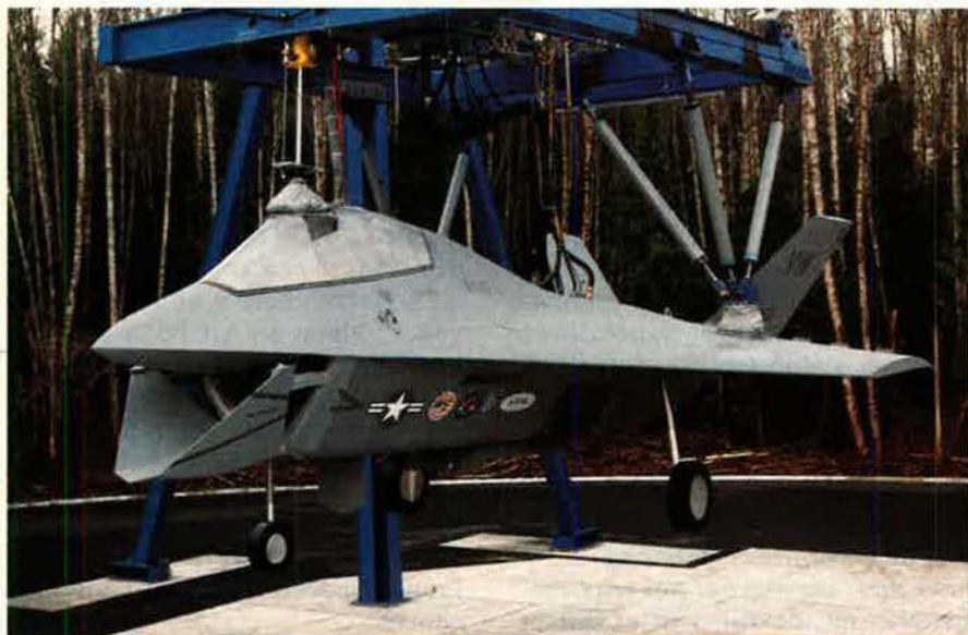
A STOVL airplane has a voracious appetite for air. Boeing's Marine version cranks its mouth open extra wide to gulp it in. The STOVL versions will handle just like the CTOL variants; controls will be "transparent" to the pilot.
