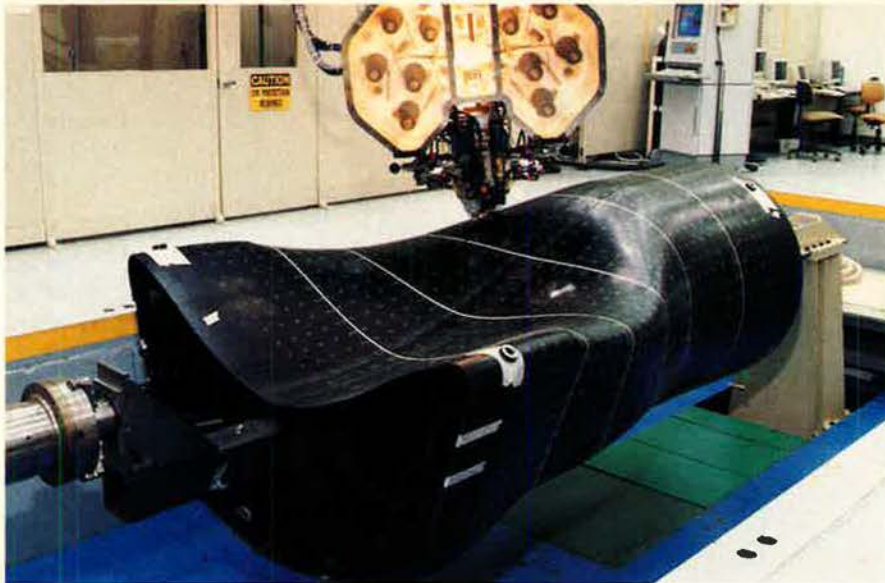
No longer just a "paper" airplane, the JSF is taking shape as a technology demonstrator aircraft. Not quite prototypes, the X-32 and X-35 will prove out flight characteristics and controls. Boeing's X-32 will use this inlet duct.
