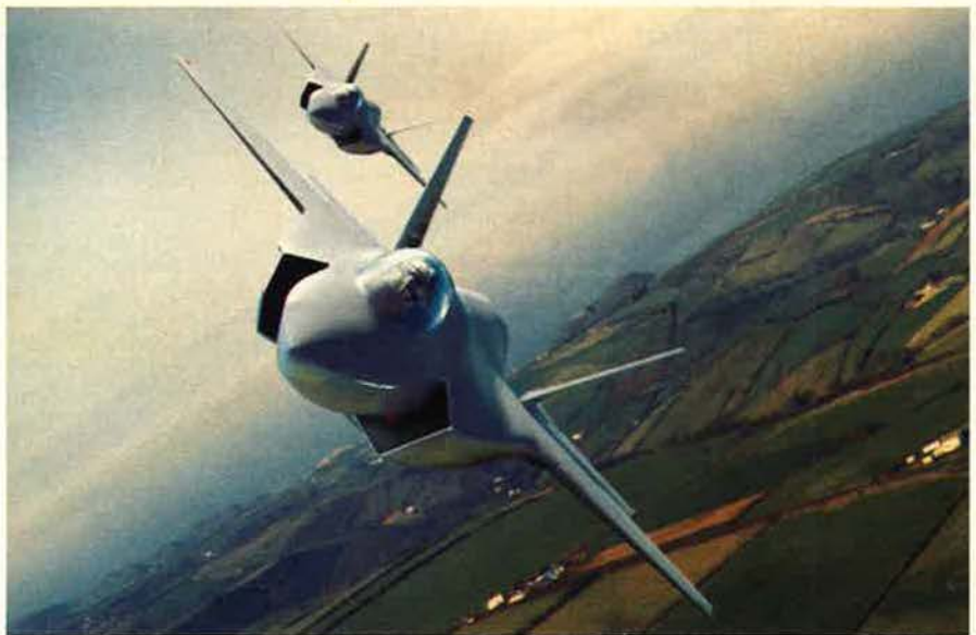
The Air Force needs 1,763 Joint Strike Fighters to replace its A-10s and F-16s. The JSF is to have better range, stealth, and reliability than the F-16 but won't necessarily be faster or more agile. Lockheed Martin's offering is shown here.
