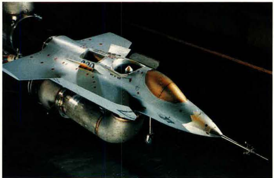
This Lockheed Martin STOVL wind tunnel model is defining the thrust generated by its lift fan concept. The lift fan, not needed for conventional takeoff, would be deleted on the USAF version and replaced by a fuel tank.
