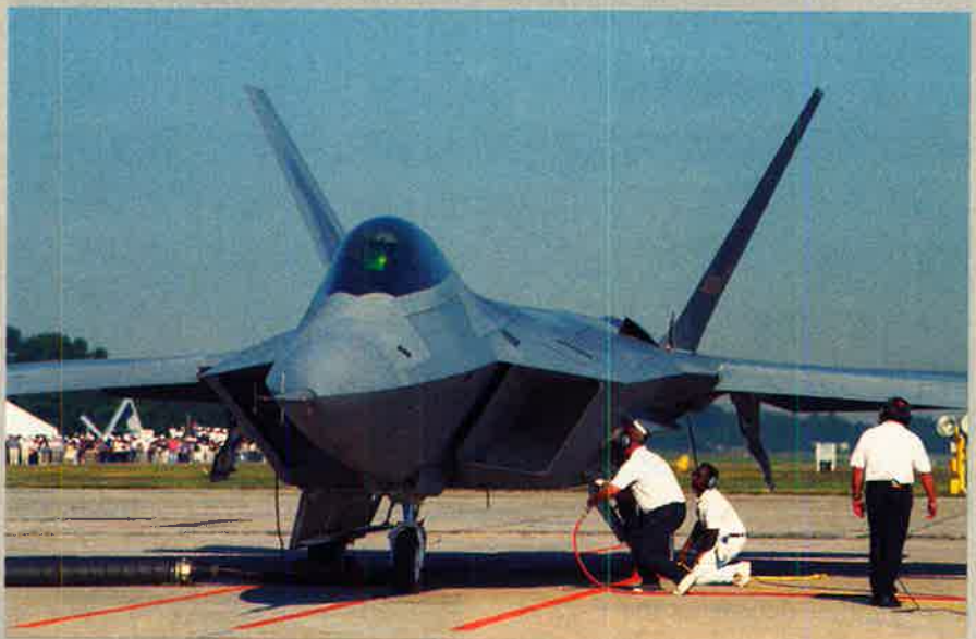
This view of the intakes shows how much the engine fan blades are shielded from radar reflection. It is one of the many characteristics that contribute to the F-22's stealth capability.
