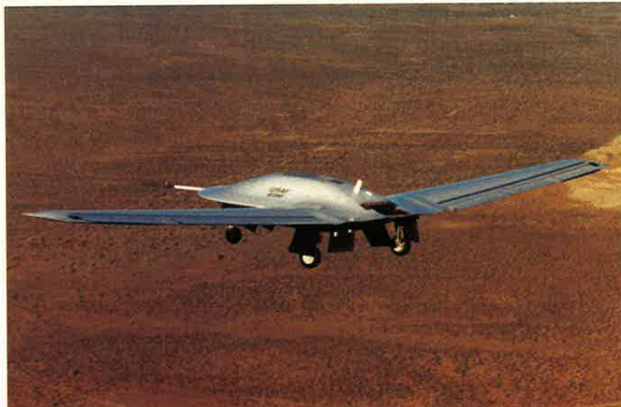
The second Tier III Minus DarkStar Unmanned Aerial Vehicle successfully completed its first flight at Edwards AFB, Calif., in June. The Lockheed Martin UAV performed a fully automated 46-minute flight, reaching 5,000 feet.
