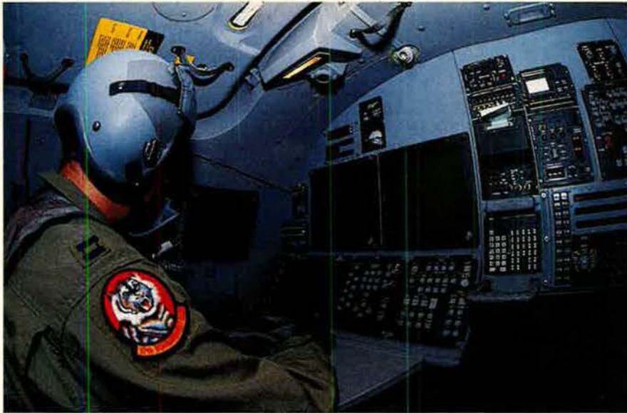
The Defensive Systems Operator suite is the focus of many upgrades. Block B improvements included the Synthetic Aperture Radar and Defensive Countermeasures System. Block F will be a Defensive Systems Upgrade.
