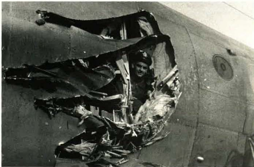
Pilot B.J. Anderson peers through the rip in his C-54's fuselage. He was taking off from Celle, Germany, when the hydraulic line to the C-54's No. 2 engine ruptured. Despite attempts to shut it down, the engine continued to accelerate and the propeller then sheared off and cut into the side of the fuselage. Anderson and his crew made a safe landing back at Celle.
