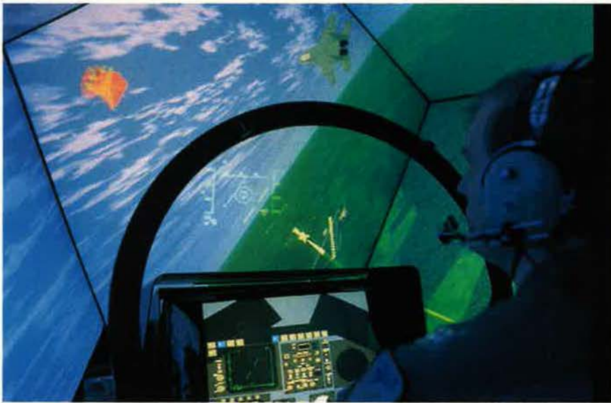
An F-22 Air Combat Simulator under development by Aeronautical Systems Center, Wright-Patterson AFB, Ohio, calls for two standard F-22 production cockpits to sit amidst 360-degree, hemispherical, visual systems capable of displaying blue sky, sun, and clouds, as well as friendly and enemy aircraft. Lockheed Martin and Raytheon are working with ASC on one such system, depicted by this graphic.
