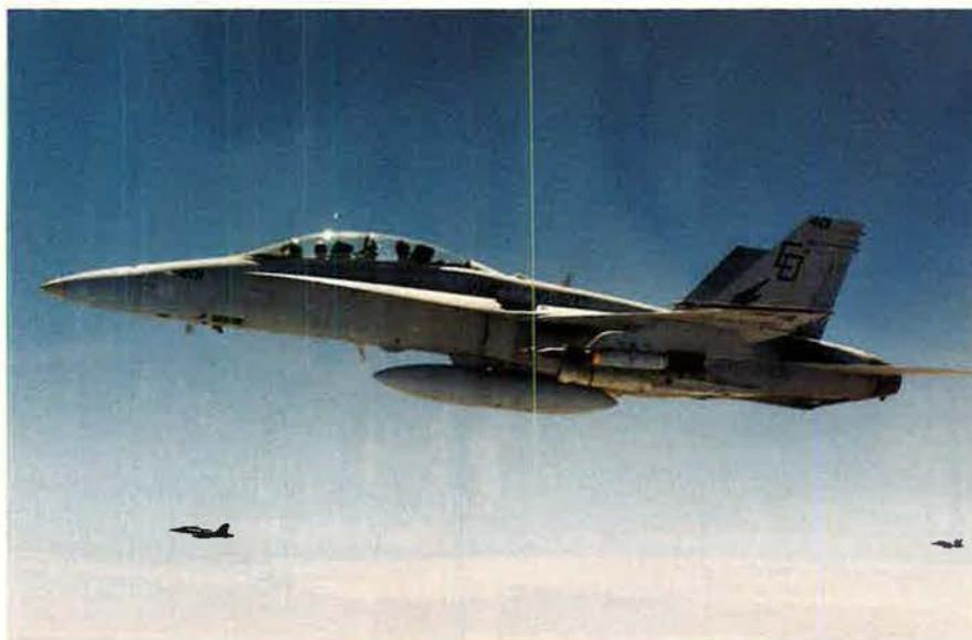
The Super Hornet is 25 percent larger than the C and D models. This two-seat F/A-18D carries a Laser-Guided Bomb on its left wing. The Super Hornet will first replace the F-14 Tomcat and then the F/A-18C/Ds.
