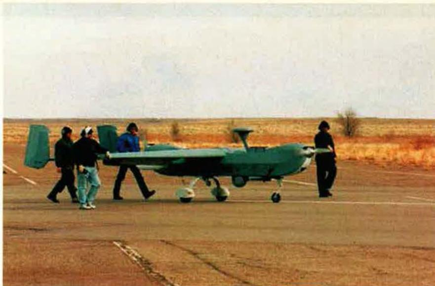
**Contract employees escort a Hunter Unmanned Aerial Vehicle to the runway at the Fort Sumner, N.M., airport, near Cannon AFB, for a test by USAF's UAV Battlelab to determine if a UAV can detect and transmit locations of enemy air defenses to fighter jets. The test was successful, according to Col. Joe Grasso, UAV Battlelab commander.**
