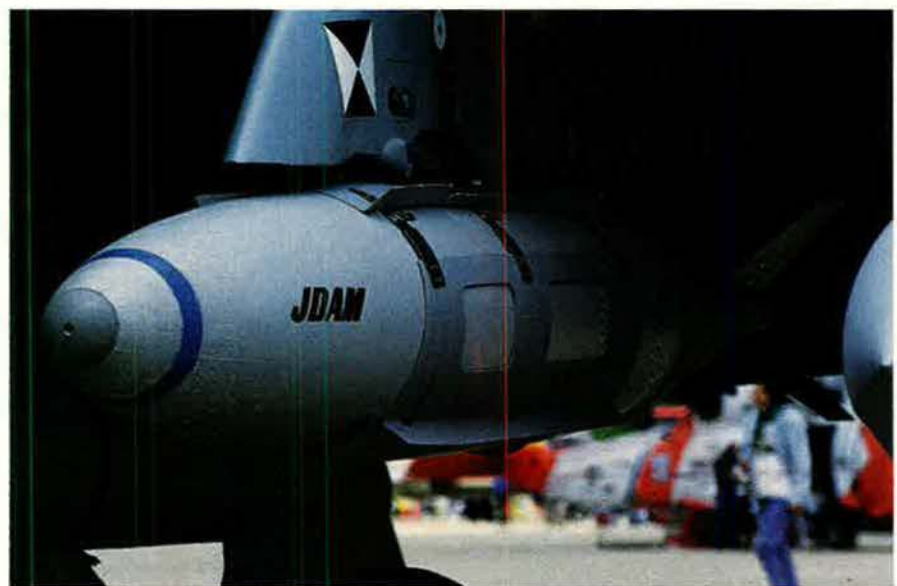
Undeterred by bad weather, JDAMs equipped with a tail kit for GPS guidance will land within 39 feet of a target. Except for the F-117, all attack aircraft will use JDAM, which comes in 1,000- and 2,000-lb versions.
