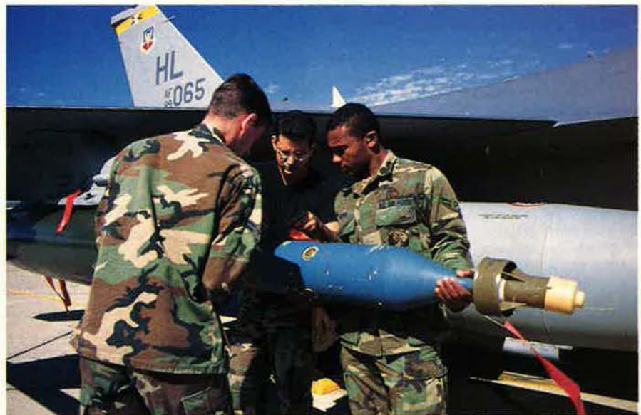
On the flight line, the weapons load crew works with the flight-line crew to load the weapon. Above, A1C Jamaal Brown drives the "jammer" as weapons load crew chief SSgt. John Barriball checks the 2,000-pound bomb. At right, once it's moved into position on the aircraft, load crew members (left to right) A1C Timothy Smith, Barriball, and Brown attach the guidance package that will turn the "iron bomb" into a GBU-24 precision guided weapon.
