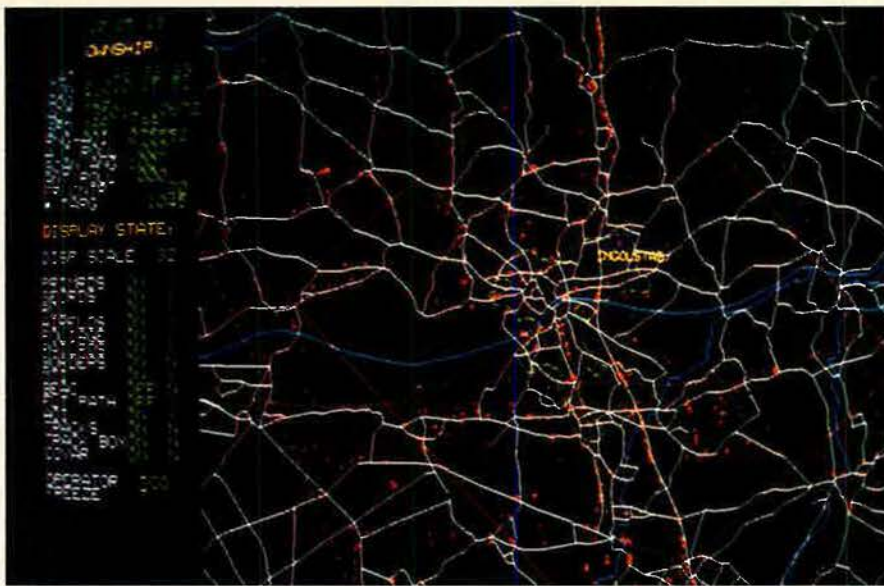
As seen in this image from an operator's console, an E-8 Joint STARS aircraft detects moving road and railroad traffic. The white lines are roads, dashed lines are railroads, blue lines are rivers, and orange dots are vehicles.
