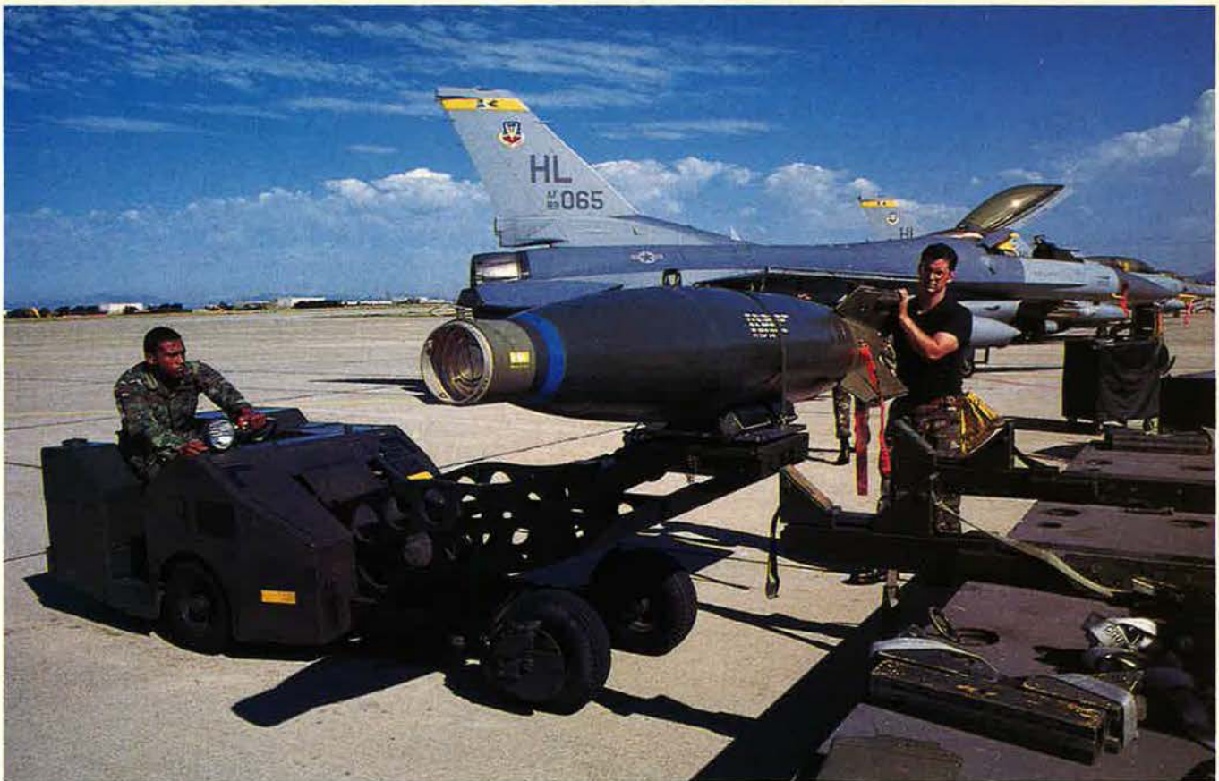
On the flight line, the weapons load crew works with the flight-line crew to load the weapon. Above, A1C Jamaal Brown drives the "jammer" as weapons load crew chief SSgt. John Barriball checks the 2,000-pound bomb. At right, once it's moved into position on the aircraft, load crew members (left to right) A1C Timothy Smith, Barriball, and Brown attach the guidance package that will turn the "iron bomb" into a GBU-24 precision guided weapon.
