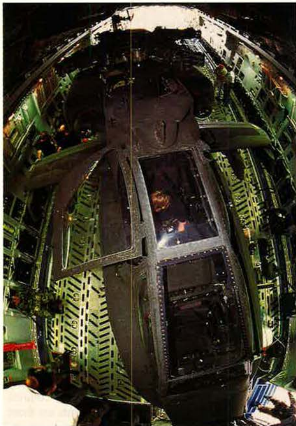
The C-17, which is larger than the C-141, can carry virtually all of the Army's air transportable outsize combat equipment. Here, with an AH-64 Apache Longbow helicopter in its cargo bay, a C-17 still has room for troops or other cargo.
