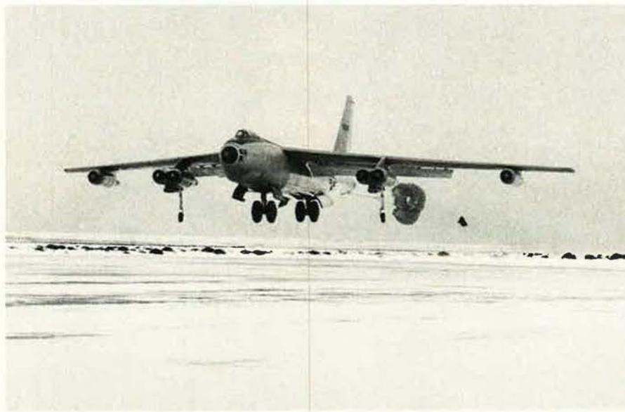
Even with landing gear and flaps down, the B-47 was so clean that it required a parachute to provide additional drag on approach. The pilot maintained power on the slow-to-accelerate jet so that a go-around could be made quickly if needed.
