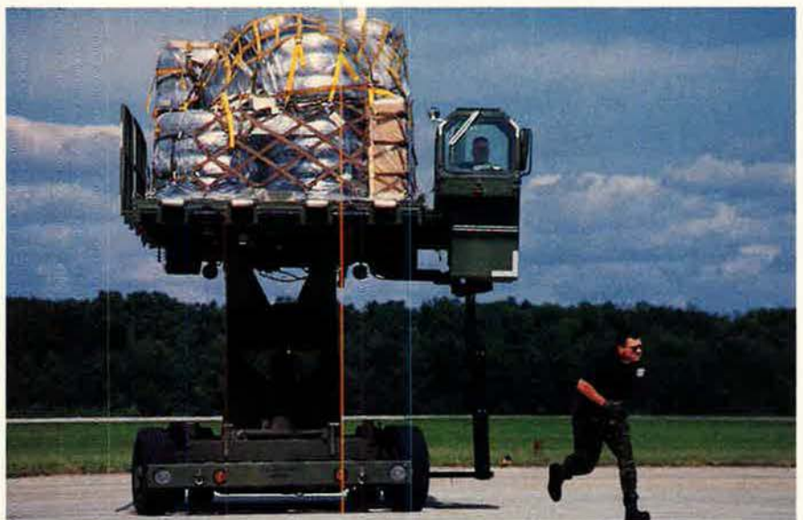
AMC is replacing old loading equipment, such as this 40K loader at Dover AFB, Del., with the new 60K loader, christened the Tunner. It will load more and heavier pallets than the 40K and doesn't need disassembly prior to airlift.
