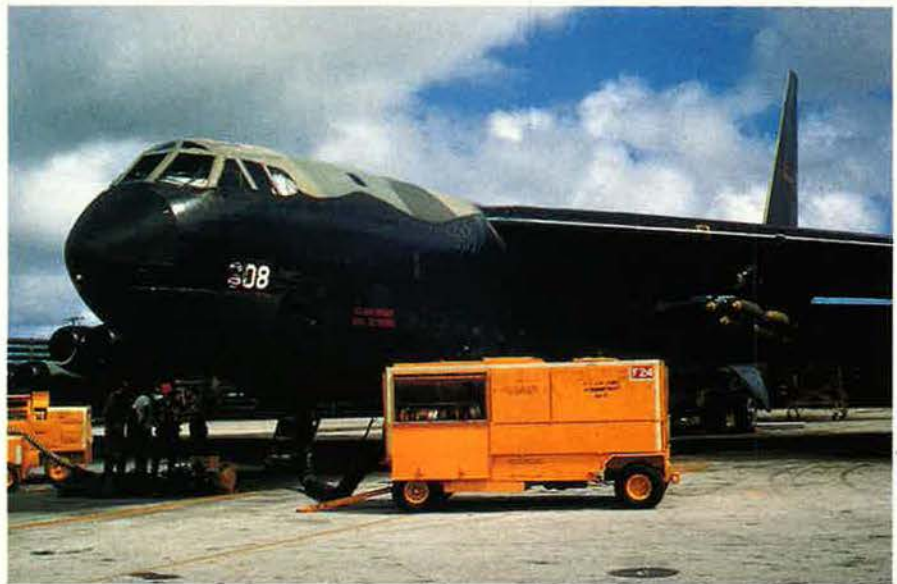
This U Tapao B-52D shows the distinctive black underside favored at the time for night missions. Clearly visible also is the left wing outboard pylon (at right in photo) loaded with extra bombs for Linebacker II missions.
