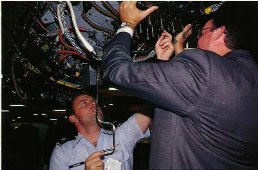
Full-scale mock-ups, like this one of Pratt & Whitney's F119 engine for the F-22, afford a unique opportunity for visitors to get "hands on" with the future. Here, Maj. Don Williams checks out the new stealth fighter engine.
