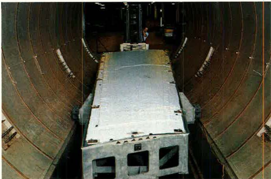
Northrop Grumman began fabrication of a new composite horizontal stabilizer for the C-17 airlifter under contract with prime contractor Boeing. The composite structure—designed to reduce weight and cost—will replace aluminum components beginning with the 51st production aircraft.
