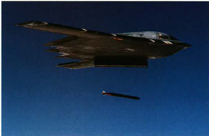
USAF continues to test various weapons with its B-2 Spirit stealth bomber, which achieved IOC April 1. In a February test, a B-2 dropped a 4,700-pound GAM-113 at China Lake NAWC, Calif. Northrop Grumman and Hughes Aircraft developed the near-precision, deep-penetration GAM-113, which the Air Force said is effective against deeply buried hard targets.
