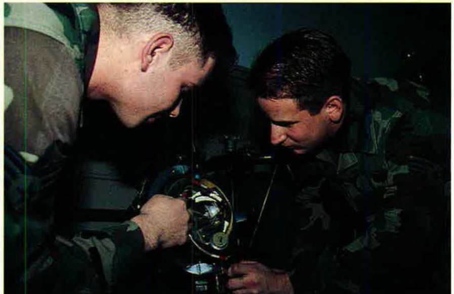
AFSPC has custody of one element of the nuclear deterrent as well as responsibility for US space-launch facilities. Here, SrA. Corey LaRock (left) and SrA. James Callari examine the forward component of a Minuteman III reentry vehicle.
